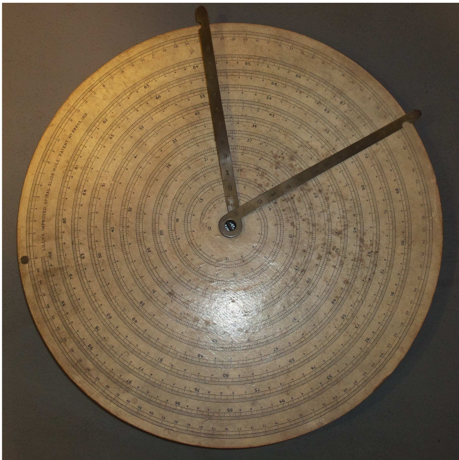
Figure 1: Lilly's improved spiral sliderule, front view
