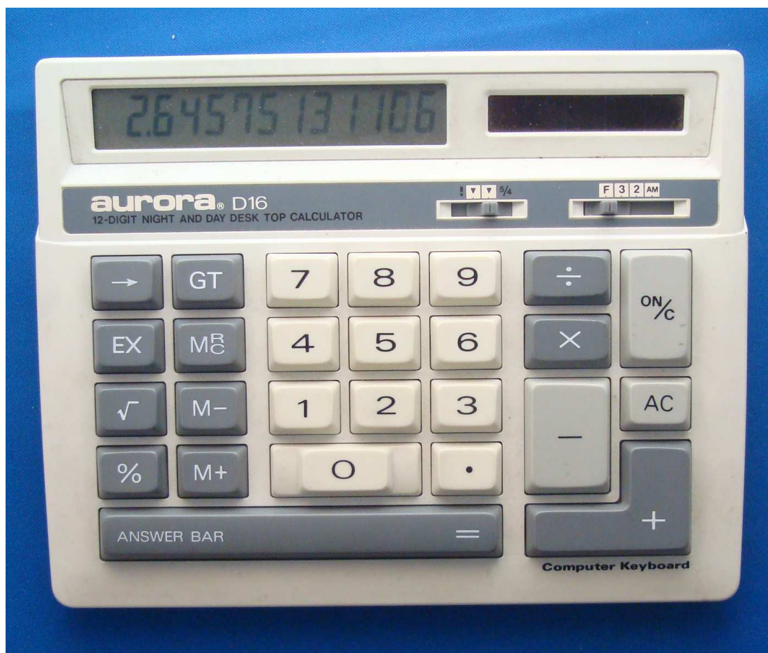
Figure 32: TCD-SCSS-U.20121208.011-fig32 Aurora D6 'Night and Day' Calculator front view Display is backlit for visibility at night
