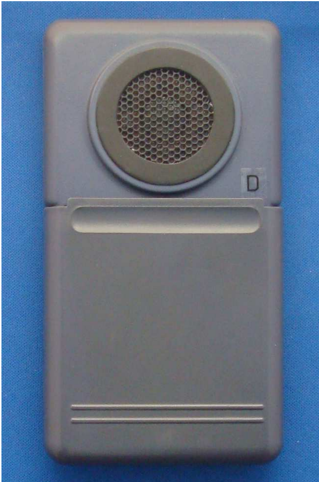
Figure 27: TCD-SCSS-U.20121208.011-fig27 Texas Instruments Pocket Dialer rear view To use, the speaker is faced towards the telephone microphone
