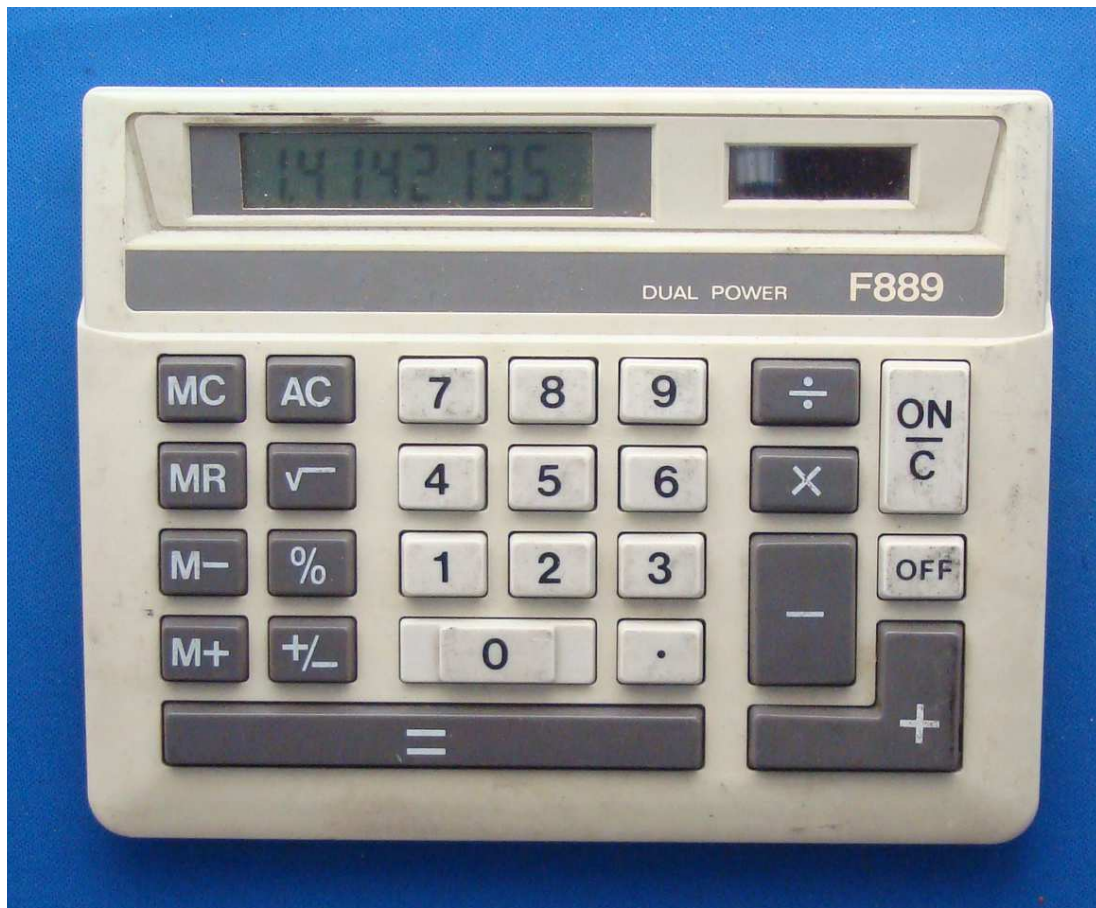
Figure 31: TCD-SCSS-U.20121208.011-fig31 F889 Dual Power Calculator front view Is powered by solar or battery
