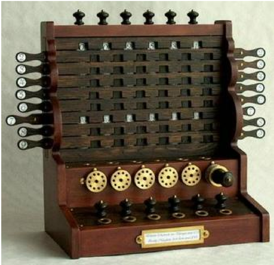
Figure 13: Reconstruction of Schickard's Calculating Clock c.1623
