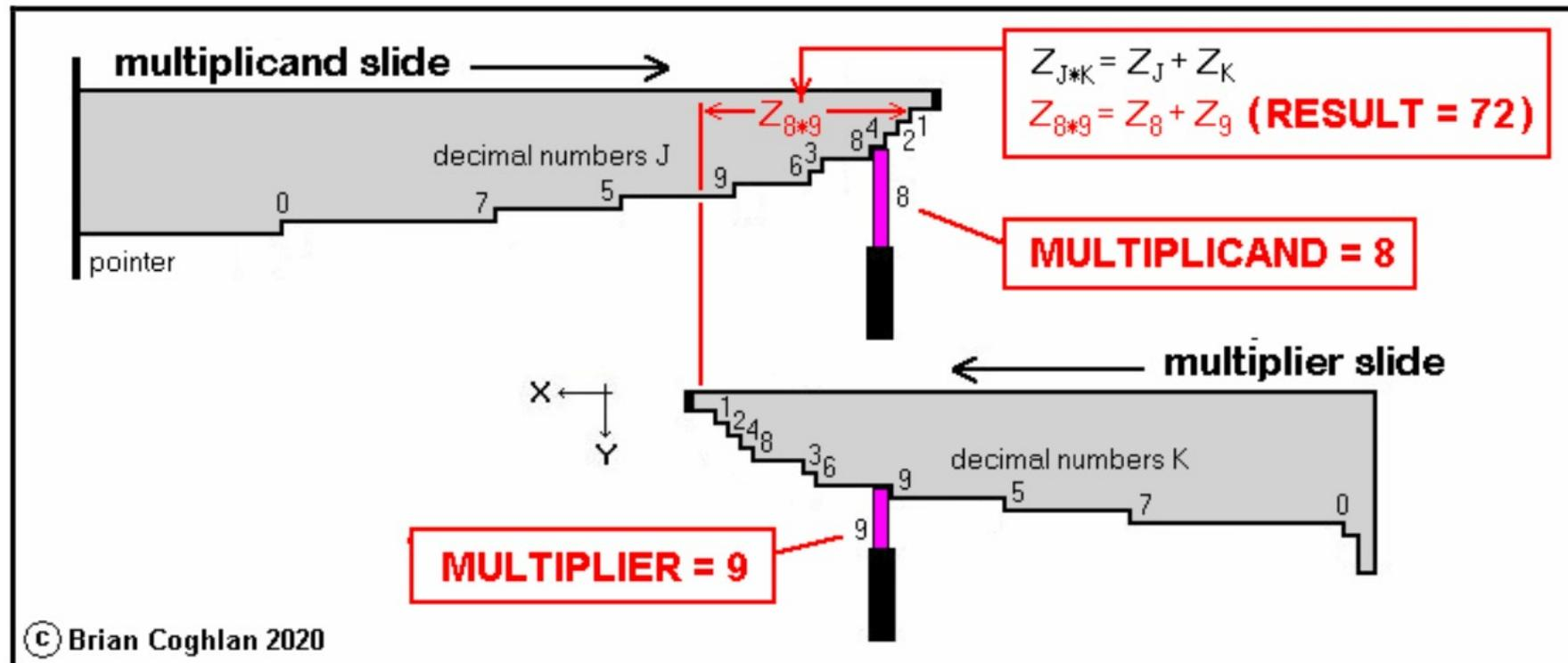
(It is not evident how the resulting product of two digits (the increased overlap of the two slides) is converted to a pair of decimal digits and transmitted to the “Mill”.)
