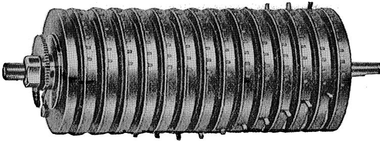
FIG. 9.—Counting Mechanism.
