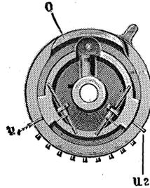
FIG. 13.—Pin Wheel of W. T. Odhner.
