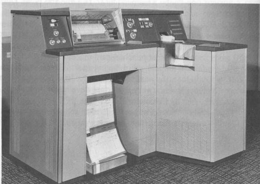
Figure 4.12. The Univac 1004 calculator, also sold in the United Kingdom and Europe as the ICT 1004, shown here, by International Computers and Tabulators (ICT, the descendant of the British Tabulating Company). Courtesy ICL Historical Collection.
