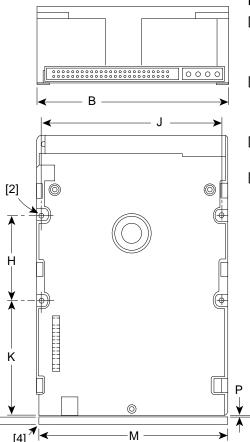
Figure 7.6-1a. Mounting configuration dimensions for "N/ND" model drives
