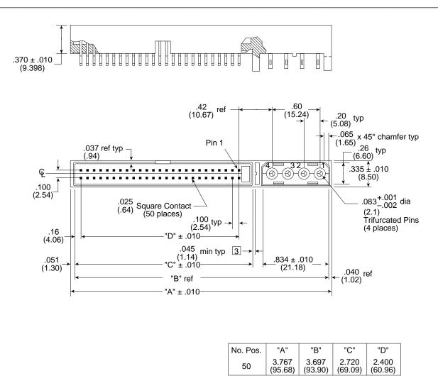
Figure 11.6.3-1a. Non shielded 50 pin SCSI device connector and 4 pin DC power drive PCB connector
