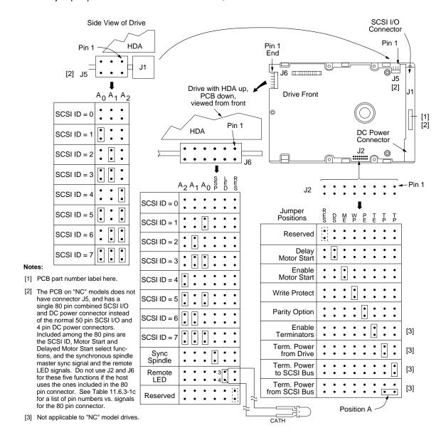
Figure 10.1-1. ST12400N/ND/NC family drive ID and option select header.
