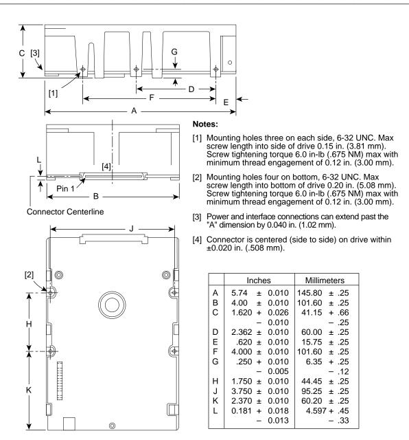
Figure 7.6-1b. Mounting configuration details for ""NC" model drives
