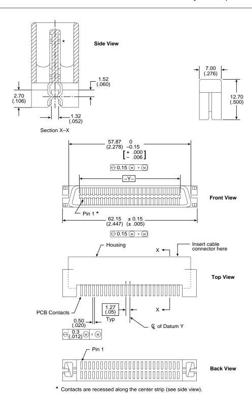
Figure 11.6.3-1b. Non-shielded 80 pin I/O and DC power connector
