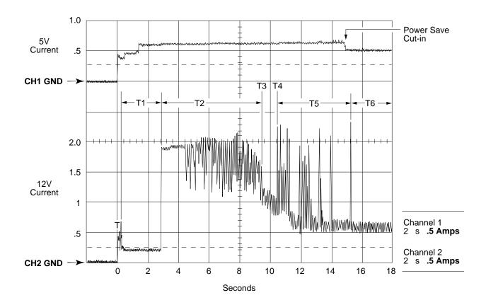
Figure 7.2.2-1. Typical Hawk 2 family drive +5 V +12 V current profile
