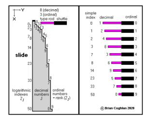
**FIGURE 4.** (Left) Ludgate's logarithmic slide, (right) shuttle rod extensions for simple indexes, decimal, and ordinal values. Image reproduced courtesy The John Gabriel Byrne Computer Science Collection.
