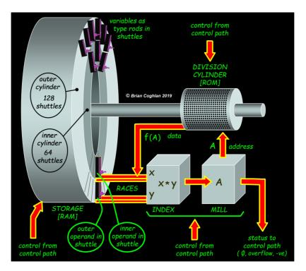
FIGURE 1. Conjectural sketch of Percy Ludgate's Analytical Machine, where "control path," "data path," "status," "RAM," "ROM," "address," "data," are modern terms, all other terms are from Ludgate's 1909 paper. Image reproduced courtesy The John Gabriel Byrne Computer Science Collection.
