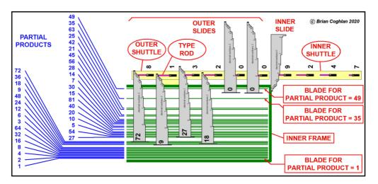
**FIGURE 6.** Ludgate's outer and inner logarithmic index slides, and inner frame with blades for compound indexes. Image reproduced courtesy The John Gabriel Byrne Computer Science Collection.
