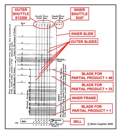
**FIGURE 3.** Annotated version of the diagram from *Engineering*, August 20, 1909, pp. 256–257.<sup>21</sup> See the Appendix for the original full-size image. Image reproduced courtesy The John Gabriel Byrne Computer Science Collection.
