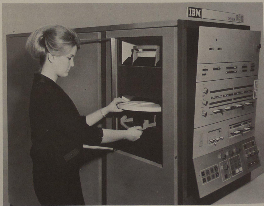
Figure 6. Removing an IBM 2315 Disk Cartridge from a Single-Disk Storage Drive
