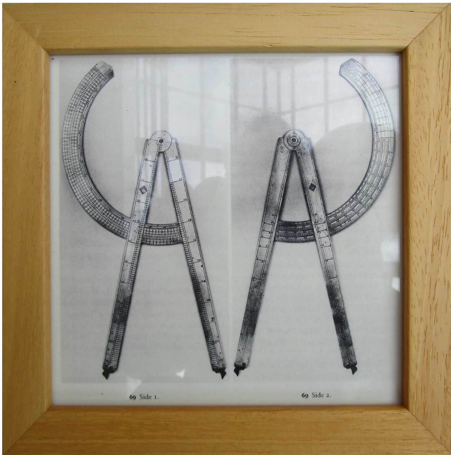
Figure 12: Illustration of both sides of a Sector
