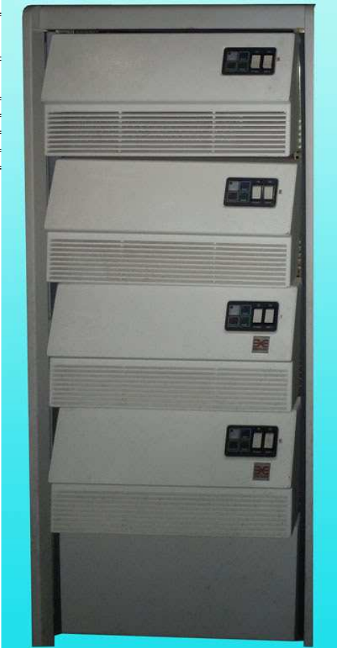
The Fujitsu Eagle SMD Disk Drives that are connected to the Emulex SC780 Controller.
