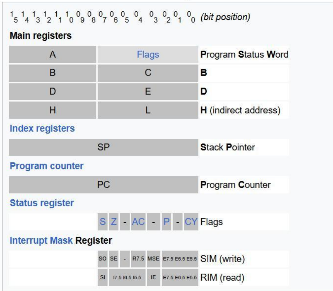
Figure 3: Intel 8085 registers (from Wikipedia).
