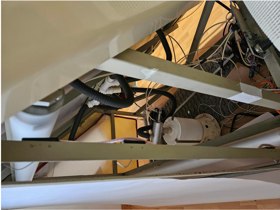
Figure 8: Sailmaking Plotter, showing vacuum pump and plumbing.
