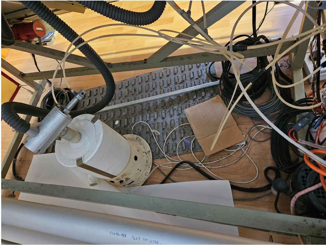
Figure 10: Sailmaking Plotter, closeup of vacuum pump.
