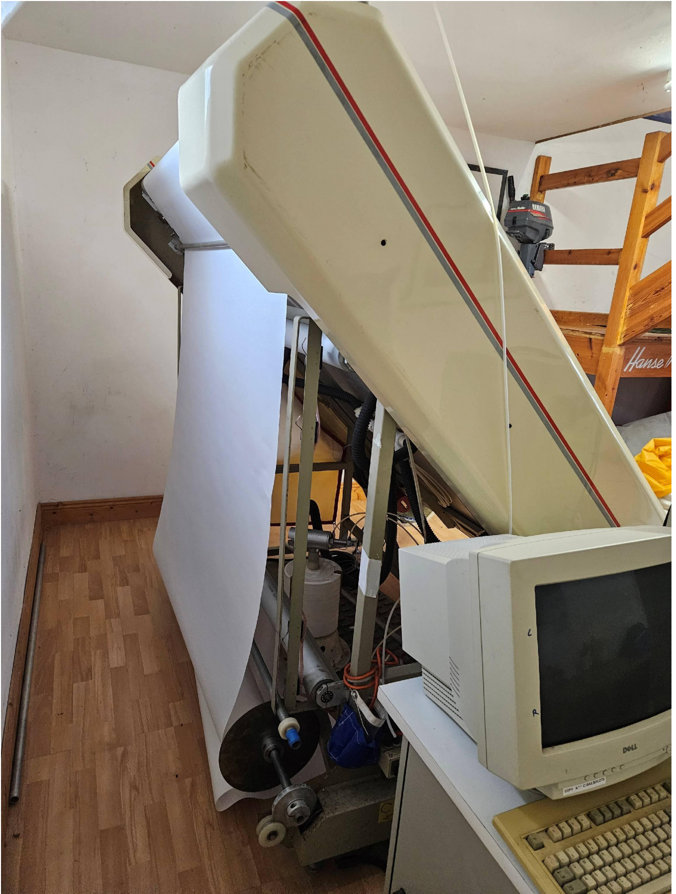
Figure 7: Sailmaking Plotter, side view showing sailcloth on servo-driven rollers.
