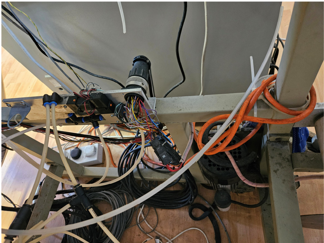
Figure 11: Sailmaking Plotter, showing wiring connections to servo-controller and position-sensing electronics.
