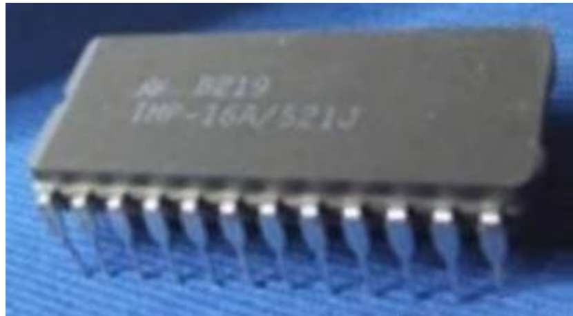
Figure 11: Top: NatSemi IMP-16 IMP-16A/521J standard control ROM (CROM).
