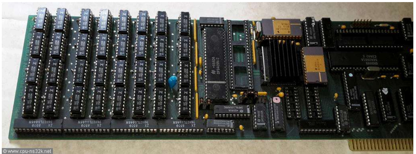
Fig. 1. The Definicon DSI-32 coprocessor board using an 8-bit ISA connector.
