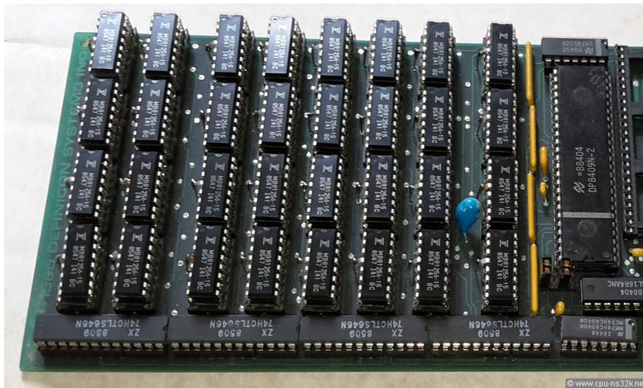
Fig. 3. A detailed look at the memory array with the memory controller DP8409N-2 on the right side.
