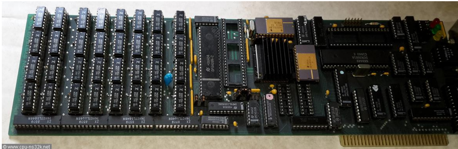
Fig. 1. The Definicon DSI-32 coprocessor board using an 8-bit ISA connector.
