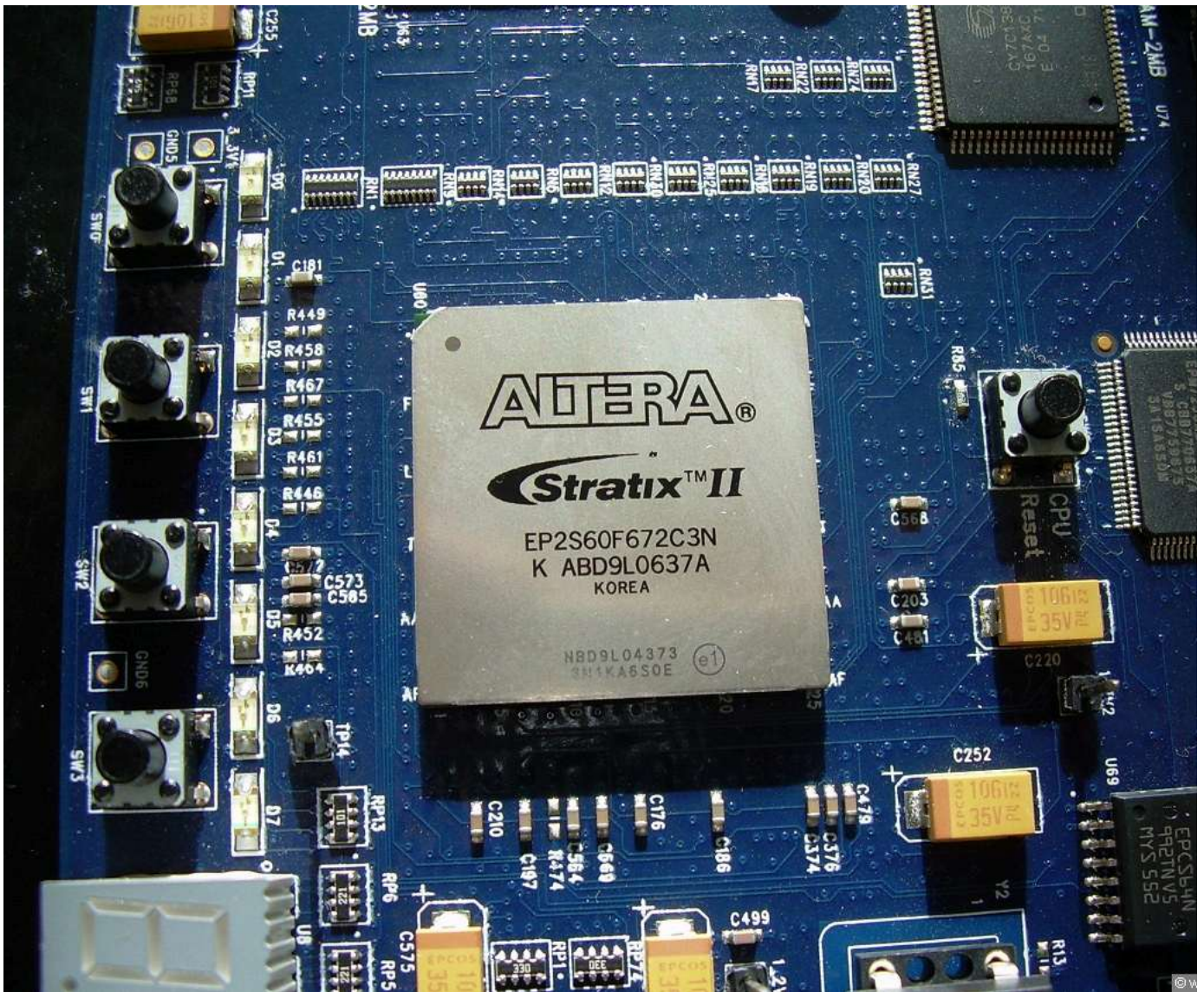
Fig. 2. The head of the system before it disappeared under the heatsink: the Stratix II FPGA. It is nice that the manufacturer went for the fastest speed grade.
