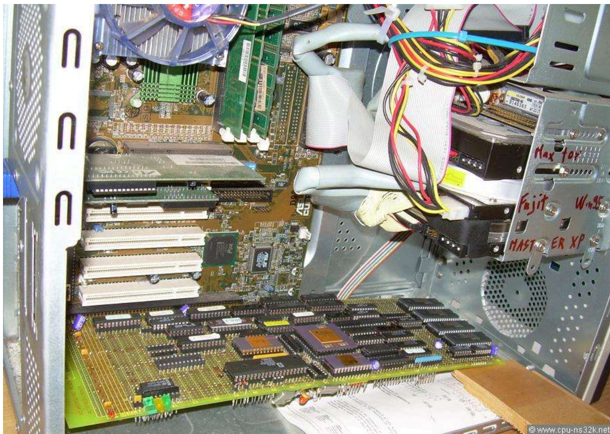
Fig. 4. Richard's coprocessor board sitting in his host system.
