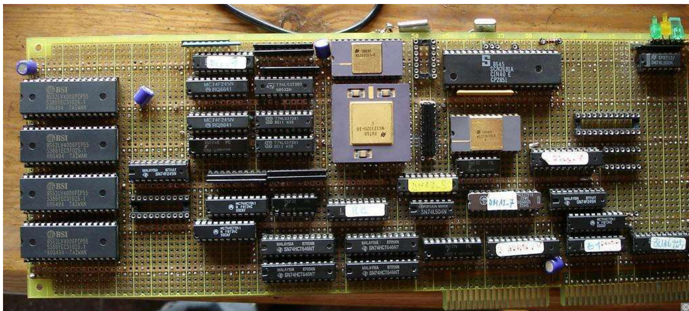
Fig. 2. Top view of Richard's coprocessor board after the SRAM upgrade.
