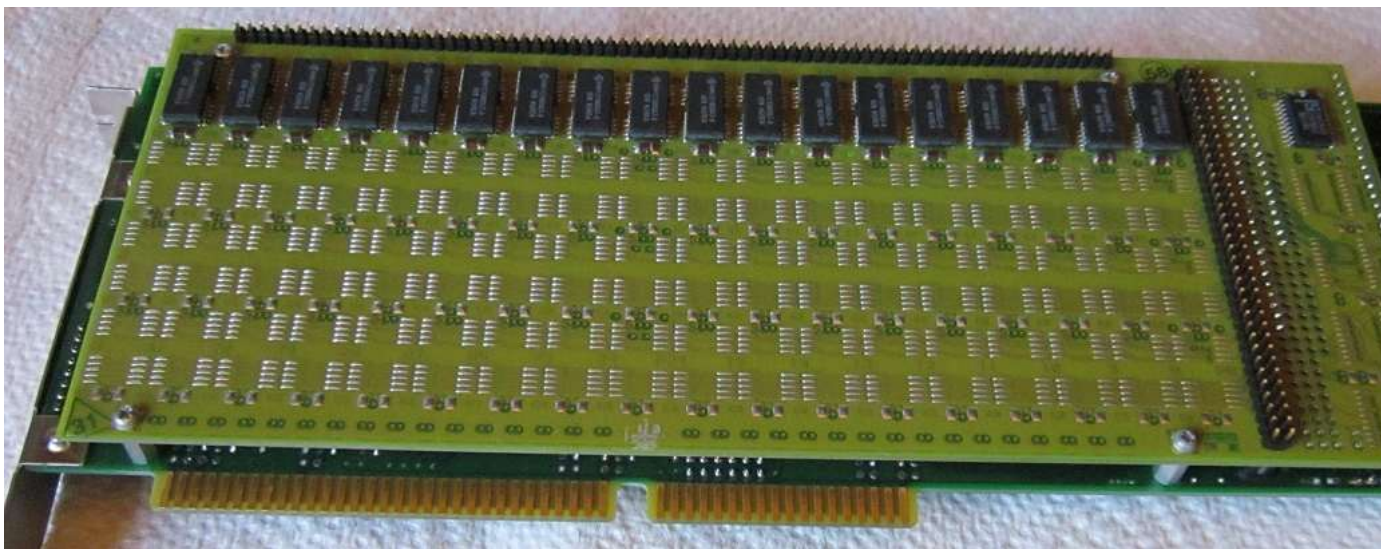
Fig. 6. A partially populated daughter board for memory expansion screwed to the CPU board.
