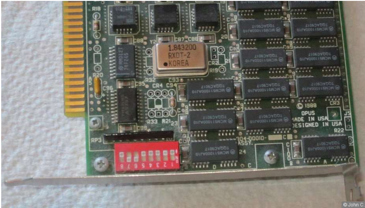
Fig. 8. The board was designed and made in the USA. Please note that the manufacturer of the DRAMs was Motorola.
