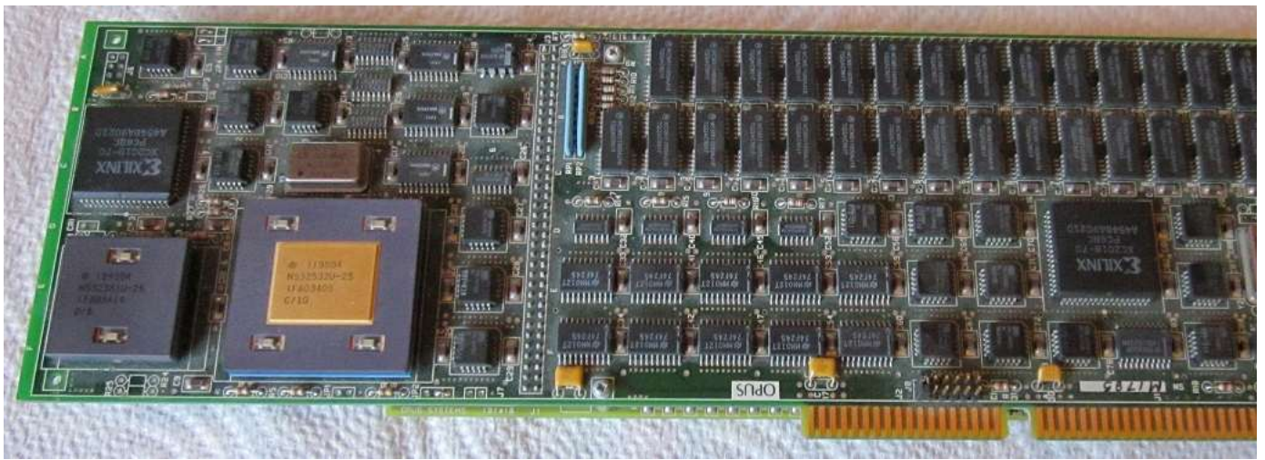
Fig. 5. The NS32532 based PC add-on board for the 16-bit ISA bus.
