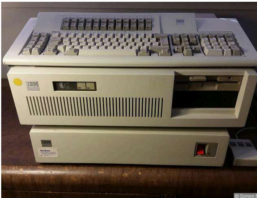
Fig. 9. Below the PC containing the Opus board is the DAU, the Display Attachment Unit.
