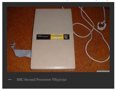
This module could plug into the back of the Acorn, and then much like the Definicon DSI-32, let Acorn users run full 32bit program on their 8bit machines. There has been an ongoing effort to emulate the Second Processor in a FPGA. Flipping that on its head, a NS32032 emulator was found, and using a FPGA Acorn, the second processor was then emulated on a raspberry pi, using a C based emulator for the NS32032.
