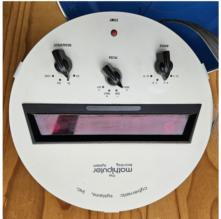
Figure 7: Cybernetic Mathiputer front panel opened, front views
