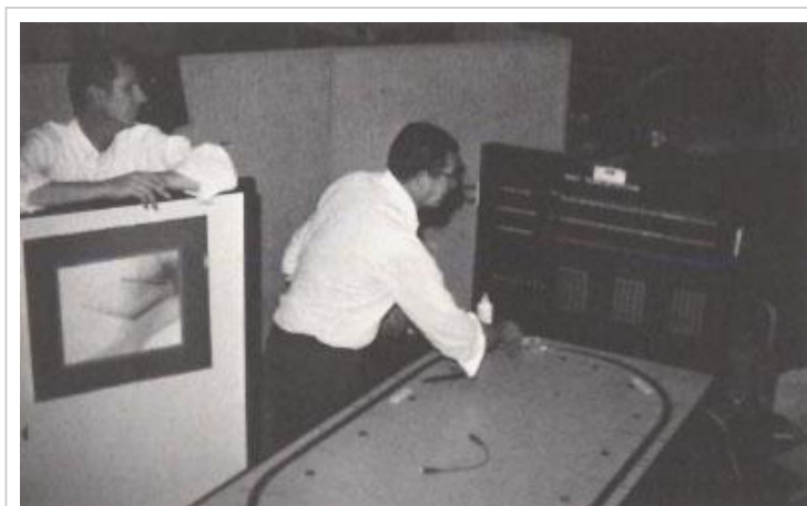
With Dave Cochran as observer, Len Cutler makes successful first test of the new train-detection system created by HP Labs team for the San Francisco Bay Area Rapid Transit District. Picture from MEASURE Magazine January 1974 Courtesy of the Hewlett-Packard Company
