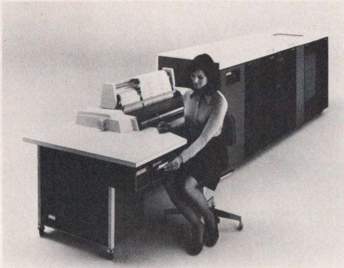
Fig. 2 — Burroughs B 721 system is designed for general purpose batch data processing.
