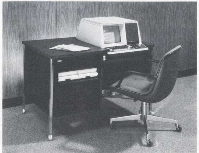
Fig. 1 — The DEC Datasystem 310 is an online small business system that includes a PDP-8/A mini with 16K characters of core memory, a VT50H or VT52 video/terminal and a dual floppy disk unit.
