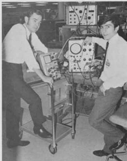
Bob Ricks and Moise Hamaoui of Instrumentation and Interface Applications investigate a problem in a phase lock loop circuit.
