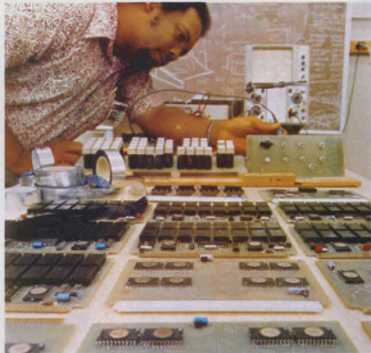
Combine an LSI microprocessor with associated circuitry and memory, and you obtain a microcomputer. In the foreground are LSI circuits and prototype systems offered by Rockwell International. The manufacturer's line includes 4 and 8-bit microprocessor chip sets.
