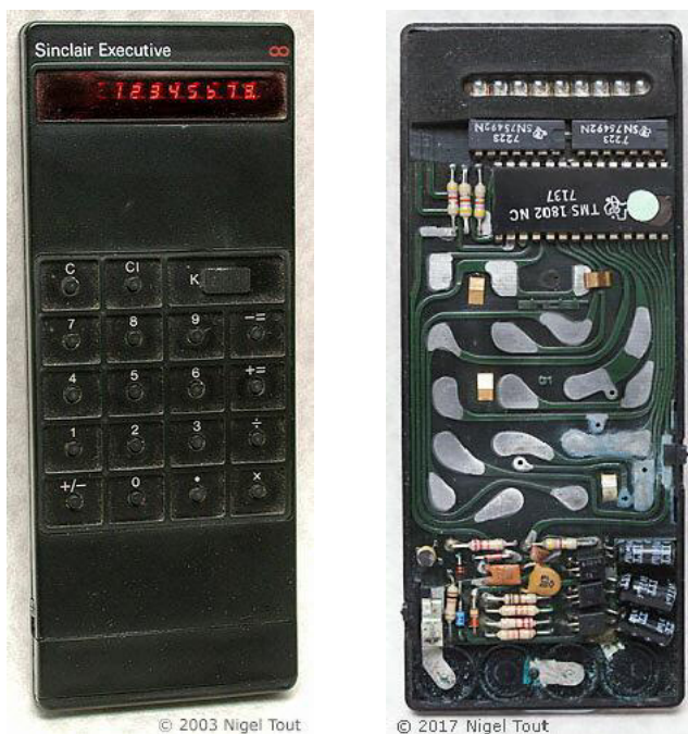
Early Sinclair Executive calculators used the TMS1802NC "calculator-on-a-chip", here date-coded to 1971, week 37. The two smaller
