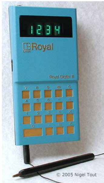
Royal Digital III , showing its unusual stylus keypad, 4-digit Vacuum Fluorescent Display (VFD), and GI 250 "calculator-on-a-chip", here date-coded to 1972, week 8.
