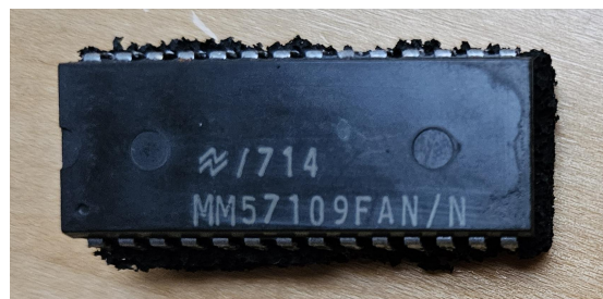
Figure 7: National Semiconductor MM57109 front view.
