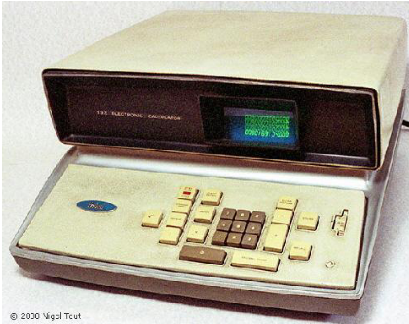
Friden EC-132 , from U.S.A., using transistors and a crt (cathode ray tube) display, 1964.
