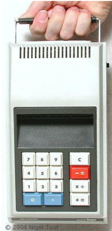
The Sharp Compet QT-8B using Rockwell-developed chips was the world's first battery-powered electronic calculator, launched in 1970.
