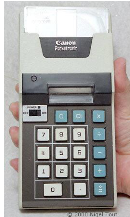
The Canon Pocketronic using chips developed by Texas Instruments was one of the first "pocket" calculators - well it would fit in a very, very large pocket. It was introduced around late-1970/early-1971.
