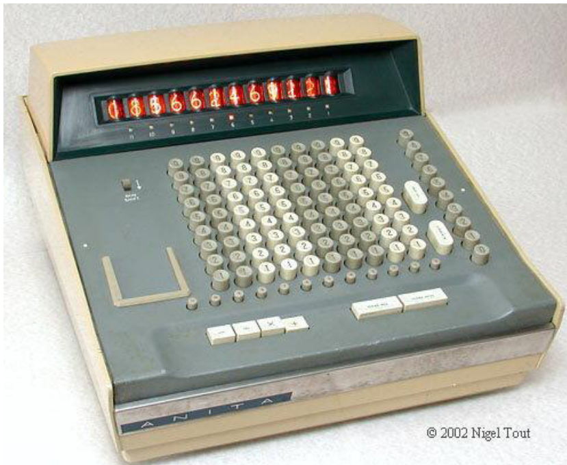
ANITA Mk 8 , from Britain, based on vacuum tube technology, 1961.
