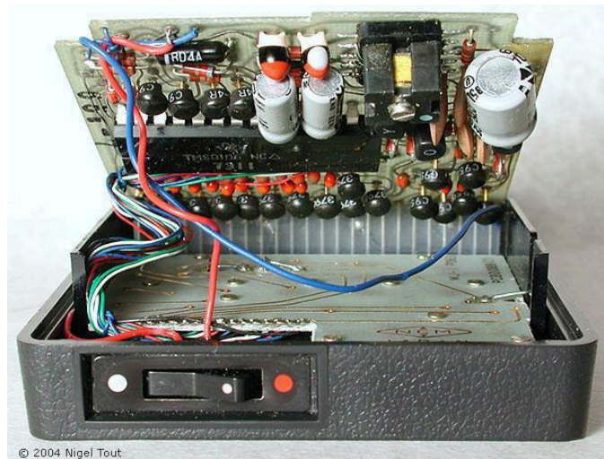
On the small circuit board in the Busicom LE-100A the black package of the Texas Instruments TMS0106 "calculator on a chip" integrated circuit can be made out on the left, behind the components at the front.
