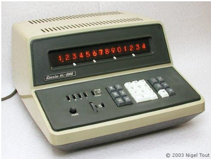
Casio AL-1000 , from Japan, using transistors, about 1967.
