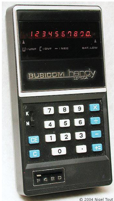
The later Busicom LE-100A "handy" pocket calculator used the Texas Instruments TMS0106 "calculator on a chip".
