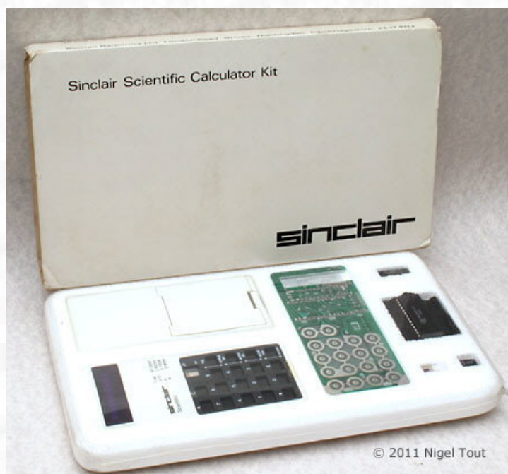
A Sinclair Scientific calculator kit, still shrink-wrapped in the polystyrene container.
