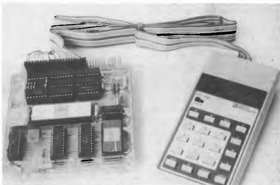
This low cost hexadecimal keyboard unit for use with the National SC/MP available from National Semiconductor.
