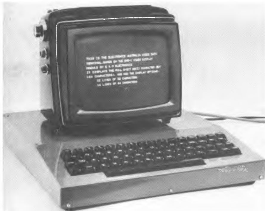
Here is the complete terminal, with a 21-cm portable TV receiver used as the display device. The low-profile case was kindly provided by Cowper Sheetmetal & Engineering, of 11 Cowper St, Granville, NSW.
