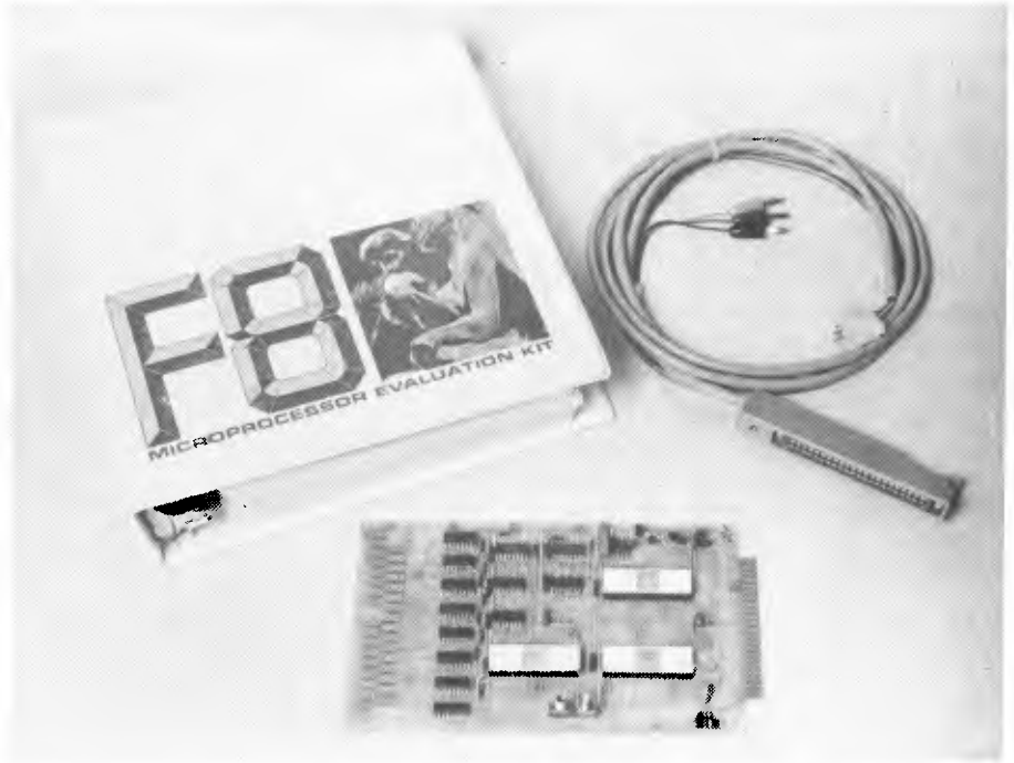
As received, the Fairchild F8 evaluation kit comprises an assembled PC board system, an edge connector with cables, and a binder of manuals.
