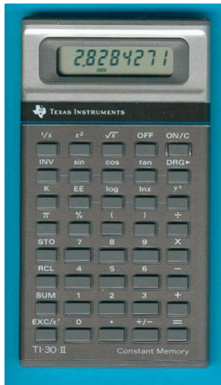
The TI-30-II calculator used the TP0320 processor. Photo courtesy of Datamath Calculator Museum .
