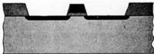
Boron is diffused, forming source and drain junctions.
