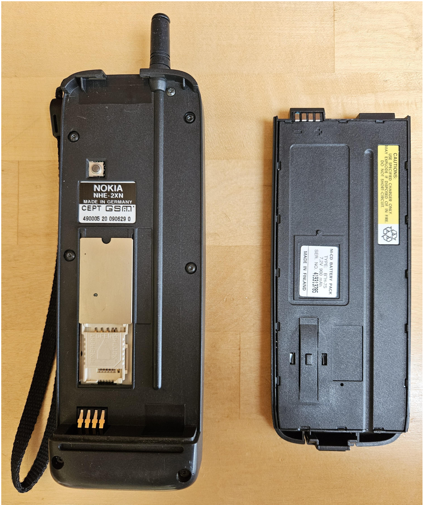
Figure 3: Left: Nokia 1011 mobile phone, rear view. “NOKIA NHE-2XN, Made in Germany, CEPT GSM, 490005-20-090629-0” Right: Nokia 1011 Battery. Rear view. “Ni-CD Battery Pack, Type BTH-7S, 7.2V 900mAh, Ser. No.: 419313785, Made in Finland”
