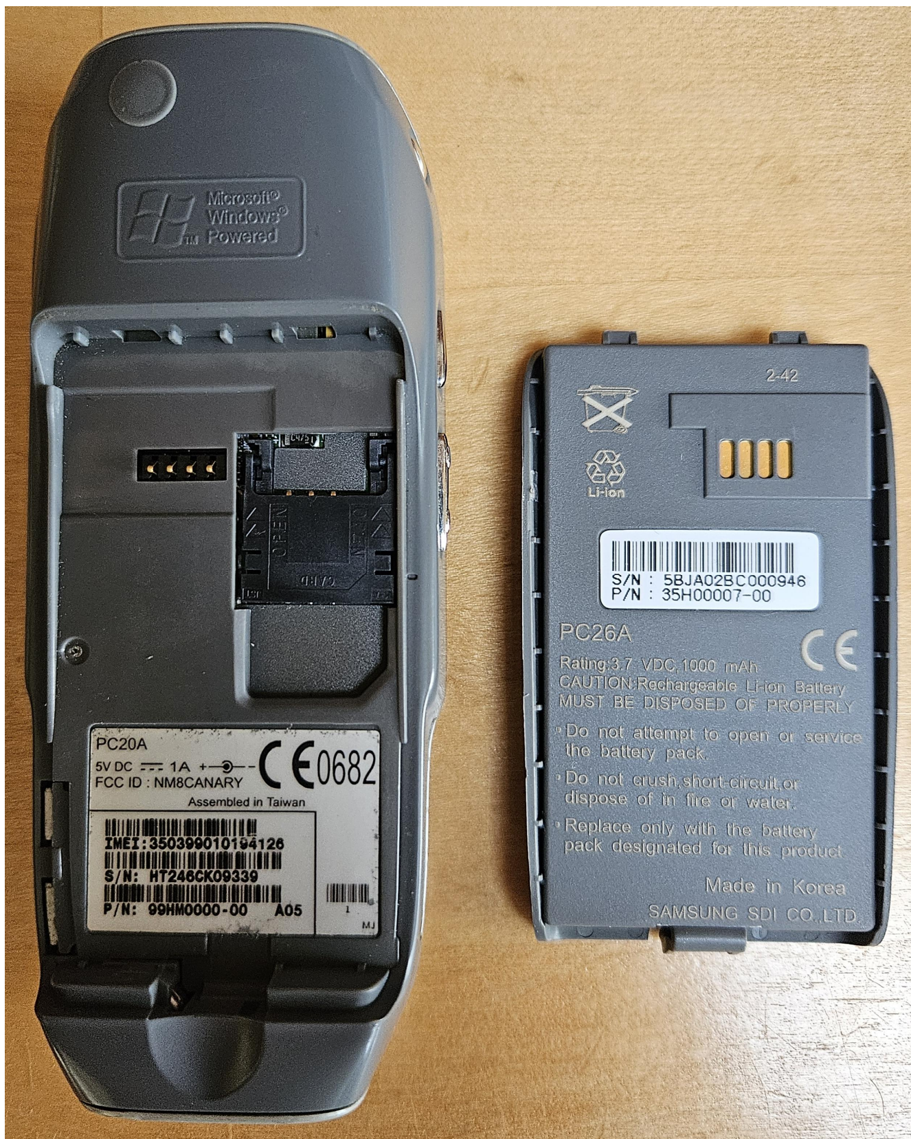
Figure 3: Orange SPV Classic manufacturing labels Mobile: "PC20A, 5V@1A, CE0682, FCC ID: NM8CANARY, Assembled in Taiwan, IMEI:350399010194126, S/N: HT246CK09339, P/N: 99HM0000-00 A05" Battery: "PC26A, S/N: 5BJA02BC000946, P/N: 35H00007-00, 3.7V 1000mAh"
