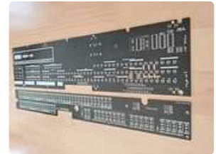
The lamp panel PCB, on top, and the separate switch panel PCB, below.
