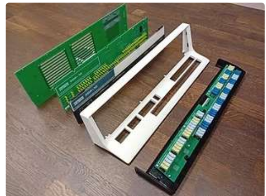
PiDP-10 parts: exploded view
