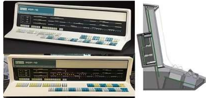
Original vs. replica: spot the difference The PiDP-10 is driven by a Raspberry Pi inside. A Pi 4 or 5 is recommended. Alternatively, work is in progress for those who prefer a plug-in FPGA simulator.
