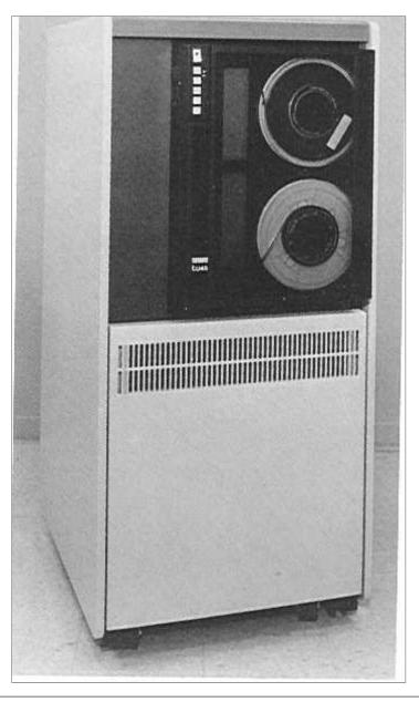
Storage medium: 1/2 inch-wide industr Capacity / tape reel: million character 40 Data transfer speed: 120000 cps at 1600 bpi Drivers/controller: 8 max Number of tracks: 9 1600 bpi or 800 bpi, p Recording density: Interrecord gap: 0.5 inch, minimum Read/write speed: 75 inch/sec Rewind speed: 250 inch/sec Rewind time: 115 sec Tape length: 2400 feet 10.5 inch Reel diameter: Max drives/system: 8 Weight per drive: 640 pounds
