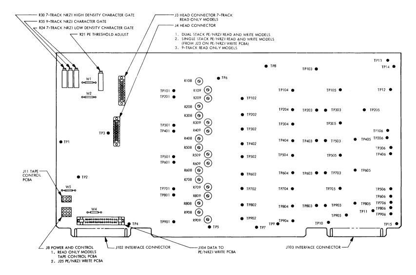
Figure 5-6. Data Kl Test Point and Connector Placement
