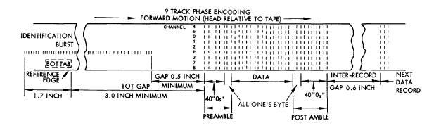
Figure 4-14. 9-Track PE Allocation and Format
