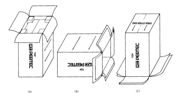
Figure 2-1. Carton Placement for Removal of Transport
