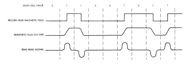
Figure 3-3. NRZI Write and Read Waveforms
