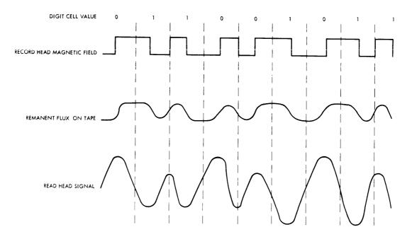
Figure 3-2. PE Write and Read Waveforms
