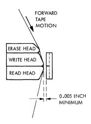
Figure 6-6. Flux Gate Adjustment
