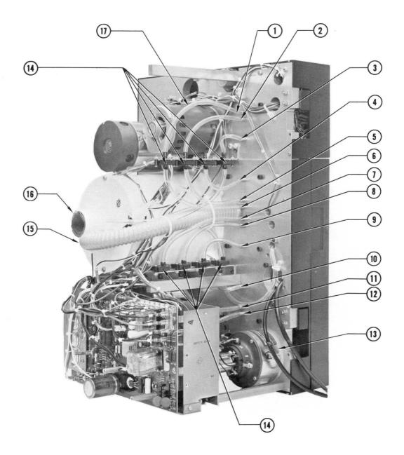
Figure 7-2. TU45 Transport Photo Parts Index, Rear View, PCBAs Removed
