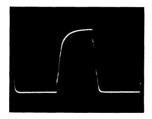
Figure 6-3. Skew Waveform (Typical)
