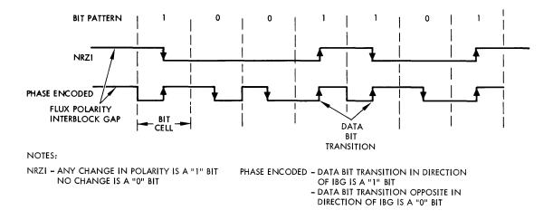
Figure 4-12. PE and NRZI Recording Comparison
