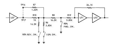
Figure 5-2. Equivalent Circuit Tape Velocity Control
