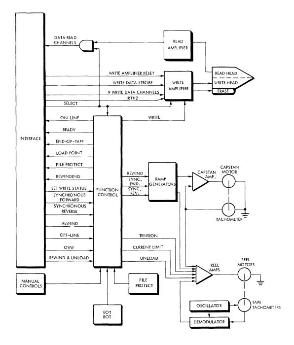
Figure 1-3. Model TU45 Tape Transport, Block Diagram
