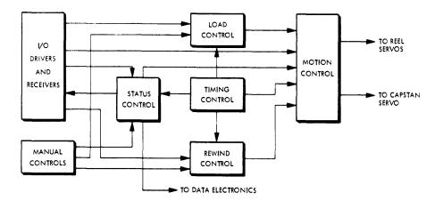
Figure 4-9. Control Logic Block Diagram
