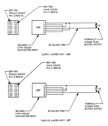
Figure 6-2. J506 and J507 Test Jumper Assemblies
