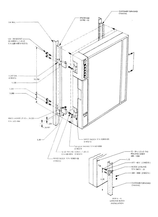
Figure 2-3. Rack Mounting the Transport
