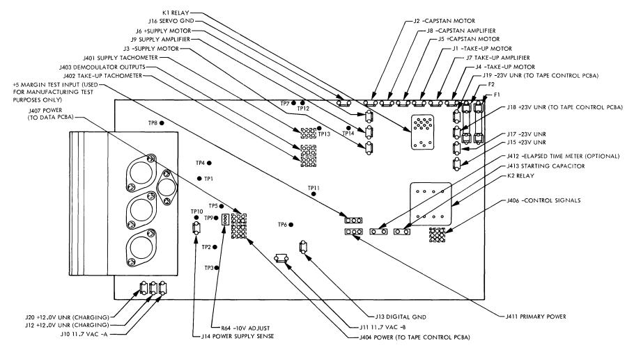
Figure 5-3. Power Supply G1 PCBA, Test Point and Connector Placement
