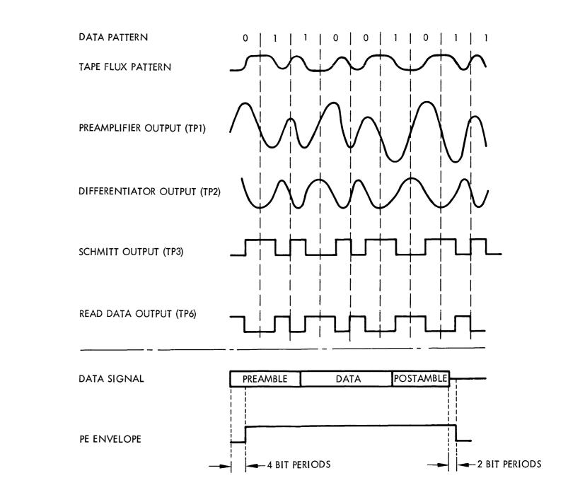
Figure 4-20. PE Data Reproduction, Timing Diagram
