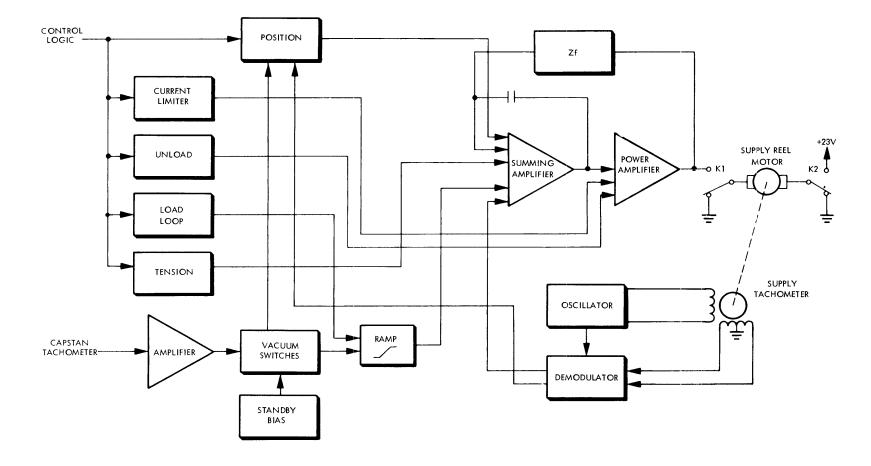
Figure 4-5. Supply Reel Servo Block Diagram
