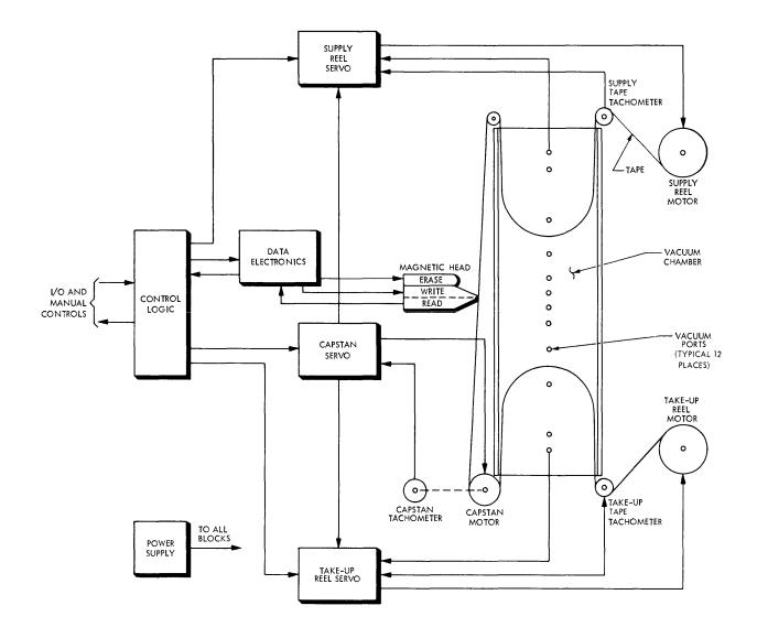
Figure 4-1. TU45 Tape Transport, Functional Block Diagram
