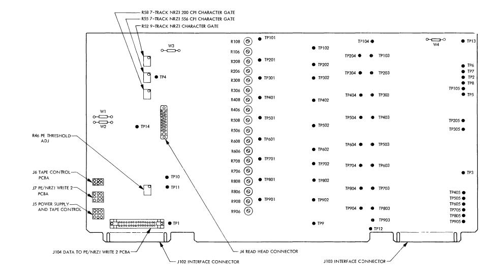
Figure 5-9. Data K2 Test Point and Connector Placement
