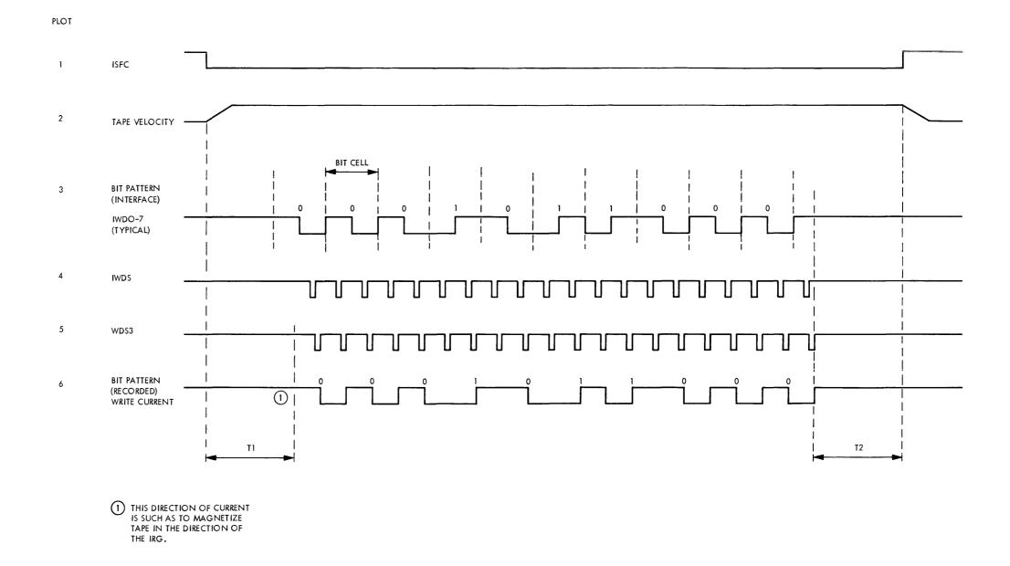
Figure 4-17. PE Data Recording, Timing Diagram
