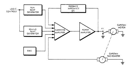
Figure 4-2. Capstan Servo Block Diagram
