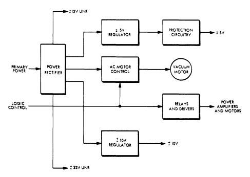
Figure 4-11. Power Supply Block Diagram
