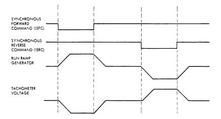
Figure 4-3. Typical Capstan Servo Waveforms
