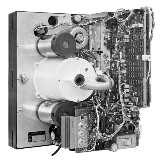
Figure 1-2. Model TU45 Tape Transport, Rear View
