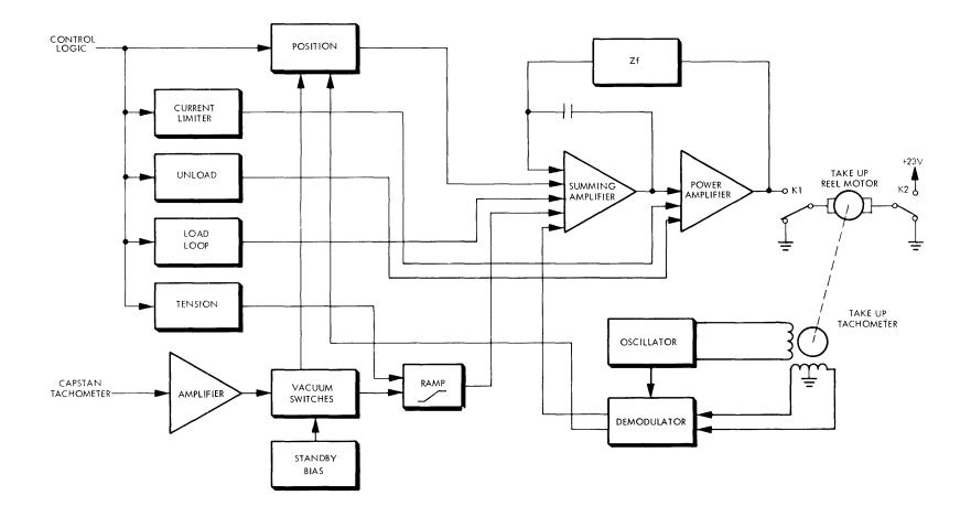
Figure 4-6. Take-up Reel Servo Block Diagram
