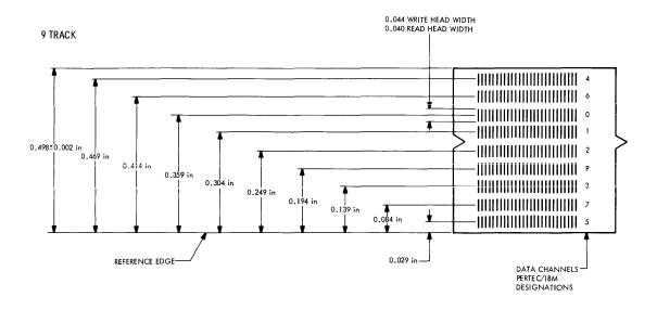
Figure 4-13. 9-Track NRZI Allocation and Spacing
