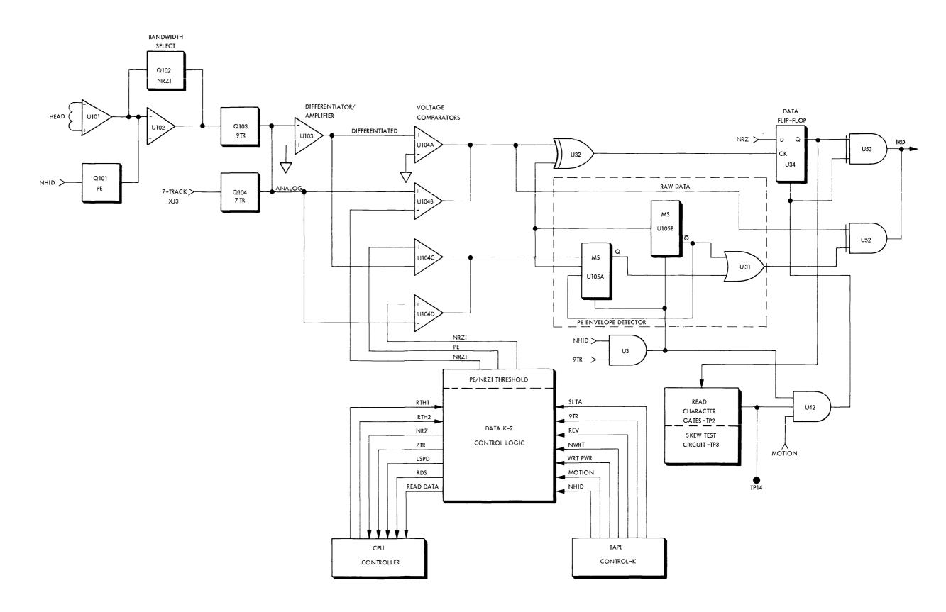
Figure 4-24. Data K2 Recovery, Block Diagram
