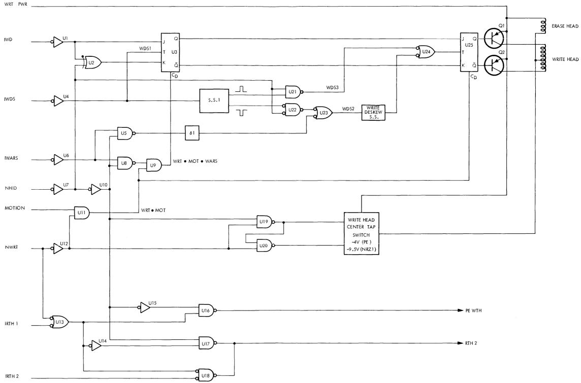
Figure 4-15. PE/NRZI Write Logic
