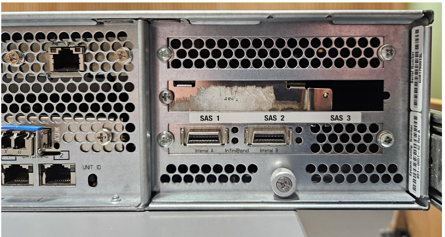
Figure 6: First Birr I-LOFAR radiotelescope on-site data acquisition computer, rear right closeup, showing internal RAID controller and 10Gbps Infiniband interface.
