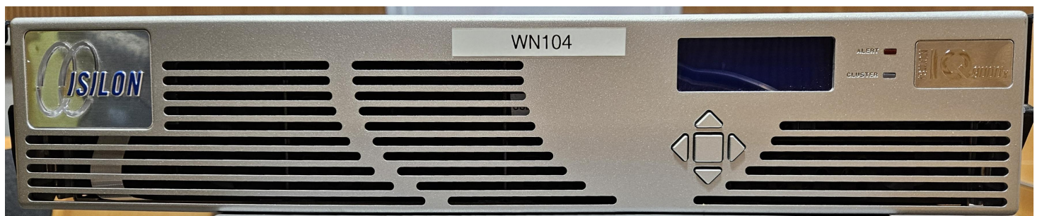
Figure 2: First Birr I-LOFAR radiotelescope on-site data acquisition computer, front view. There are twelve removeable terabyte-scale SATA RAID drives behind the removable front panel.
