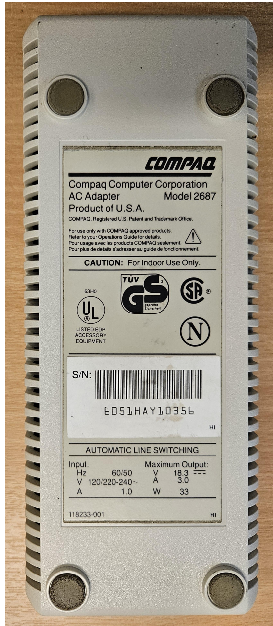
Figure 13: Compaq SLT 386s/20 AC Adaptor, top views, and manufacturing label. “Model: 2687, S/N: 6051HAY10356”.
