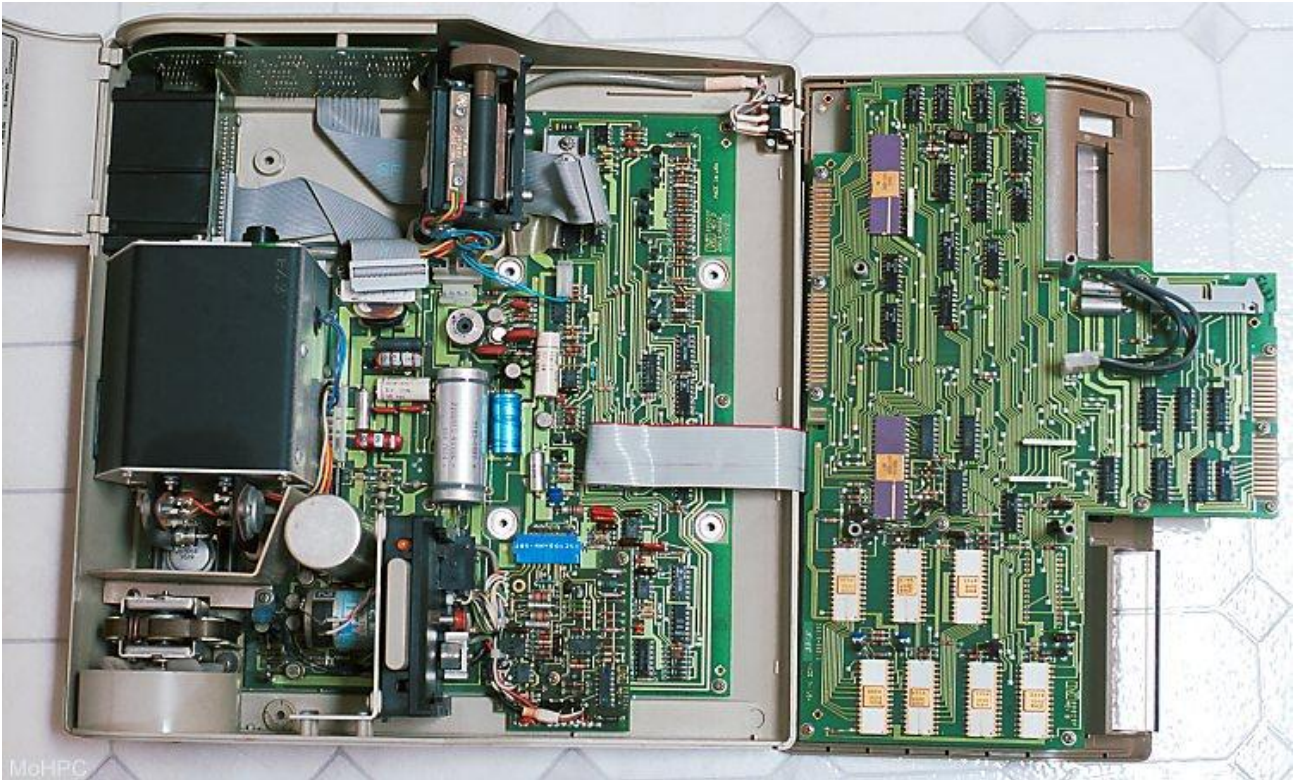
Figure 11: HP9815A calculator, internals, top view. From https://www.hpmuseum.org/hp9815.htm .
