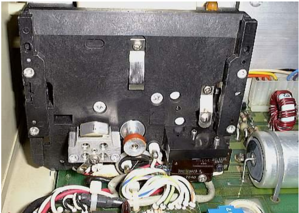
Figure 12: HP9815A calculator, tape drive mechanism. From https://www.hpmuseum.org/hp9815.htm .
