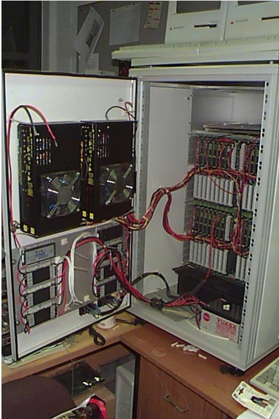
Figure 6: Orla-I dual-redundant power supply.
