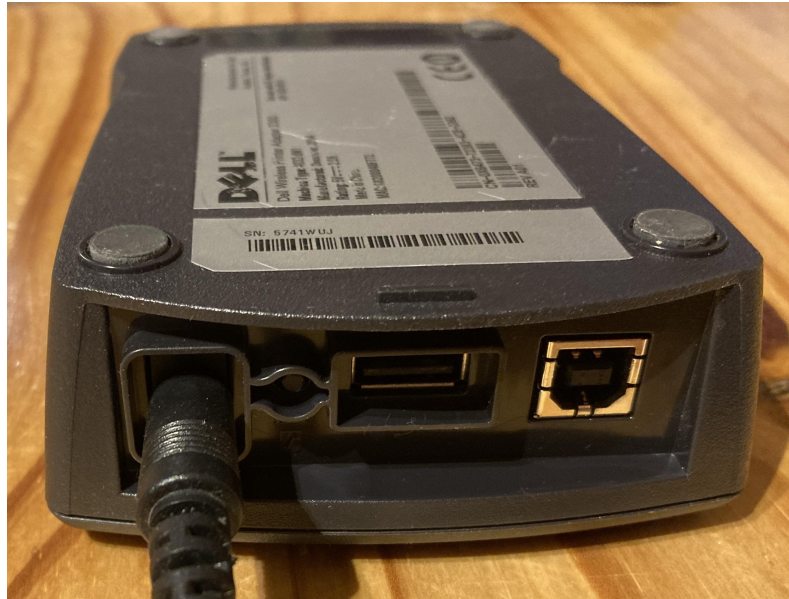
Figure 4: Dell 3300 Print Server, side view, showing left USB connector for setup, and right USB connector for connection to printer
