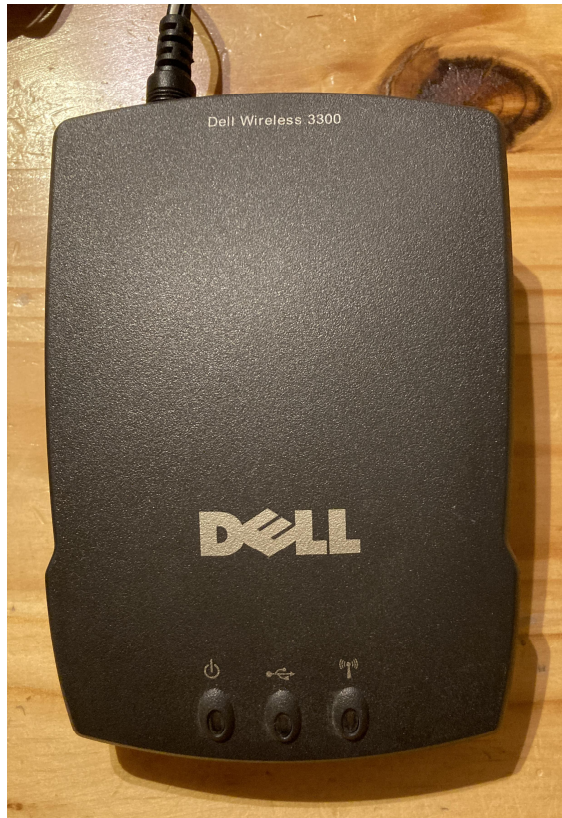
Figure 2: Dell 3300 Print Server, closeup top view LEDs indicate (left to right): power, printer activity, WiFi activity
