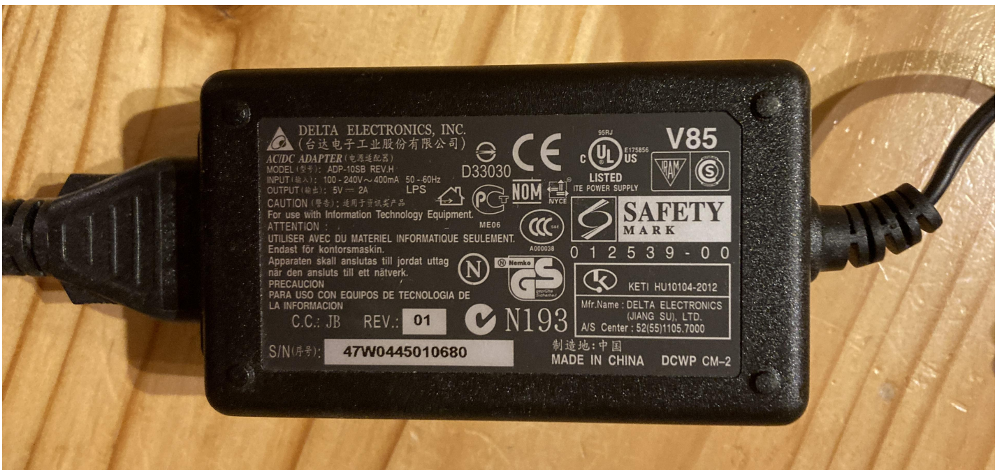
Figure 5: Dell 3300 Print Server, power supply, showing manufacturing label S/N: 47W0445010680
