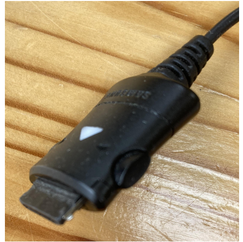
Figure 10: Samsung SGH-ZV10 USB data link cable, with closeup of Samsung proprietary male plug
