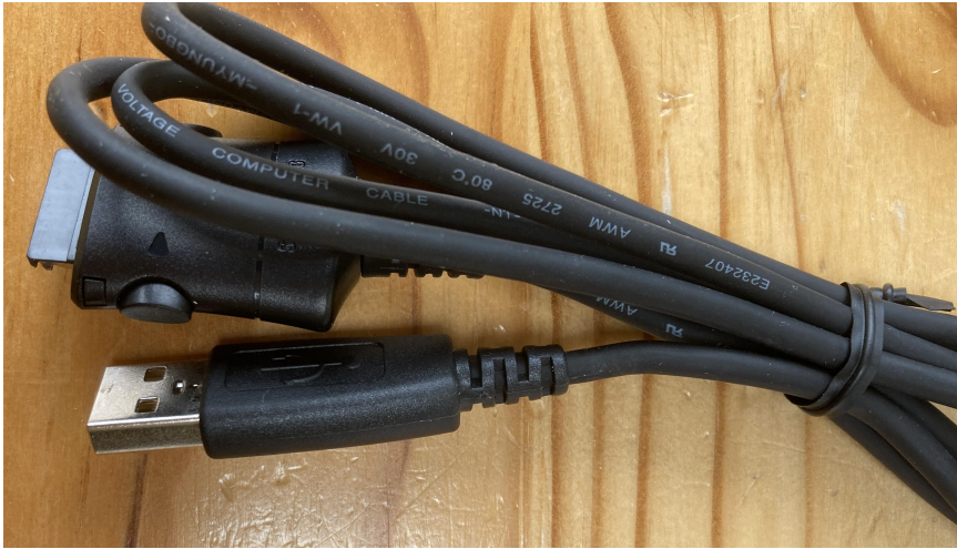
Figure 10: Samsung SGH-ZV10 USB data link cable, with closeup of Samsung proprietary male plug
