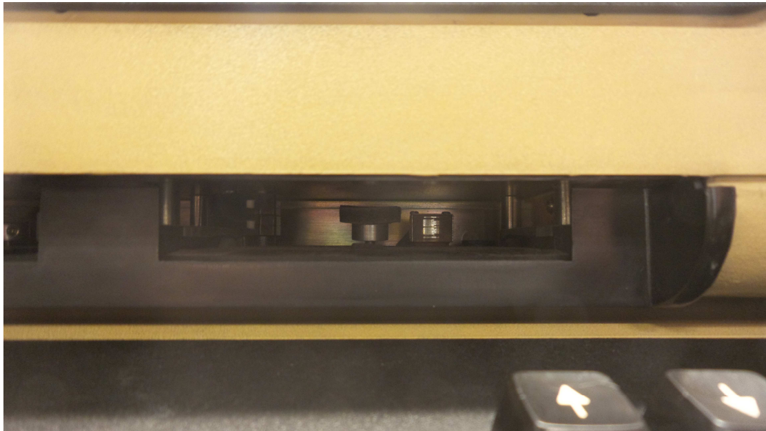
Figure 11: VT103 right TU58 DECtape-II tape heads
