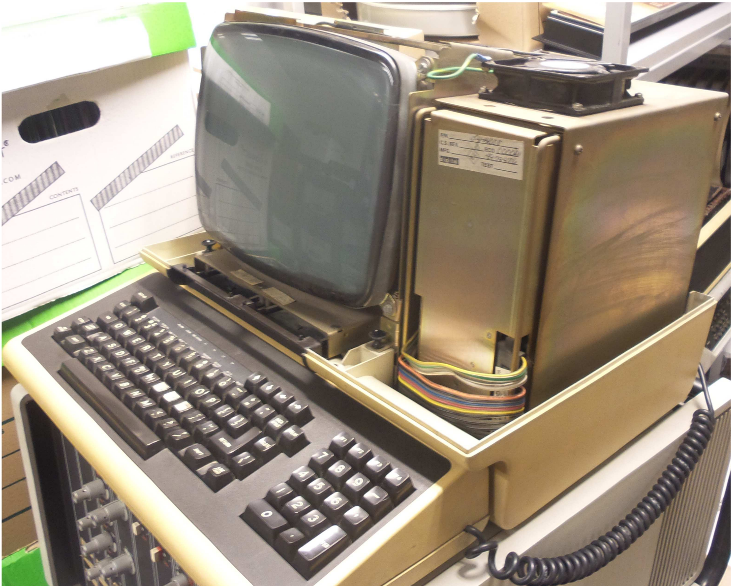
Figure 3: VT103 front three-quarter view without top cover
