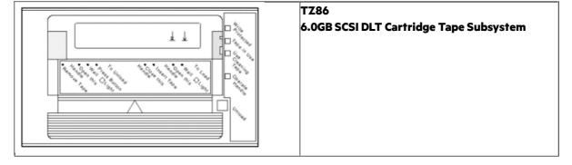
The TZ86 series of cartridge tape subsystems are used primarily as backup storage devices and as devices for loading software onto Digital computer systems. The TZ86 comes embedded in a system enclosure or in a tabletop enclosure with its own power supply. The TZ86 drive is a streaming tape drive that can store up to 6.0 gigabytes of data on a CompacTape III cartridge.
