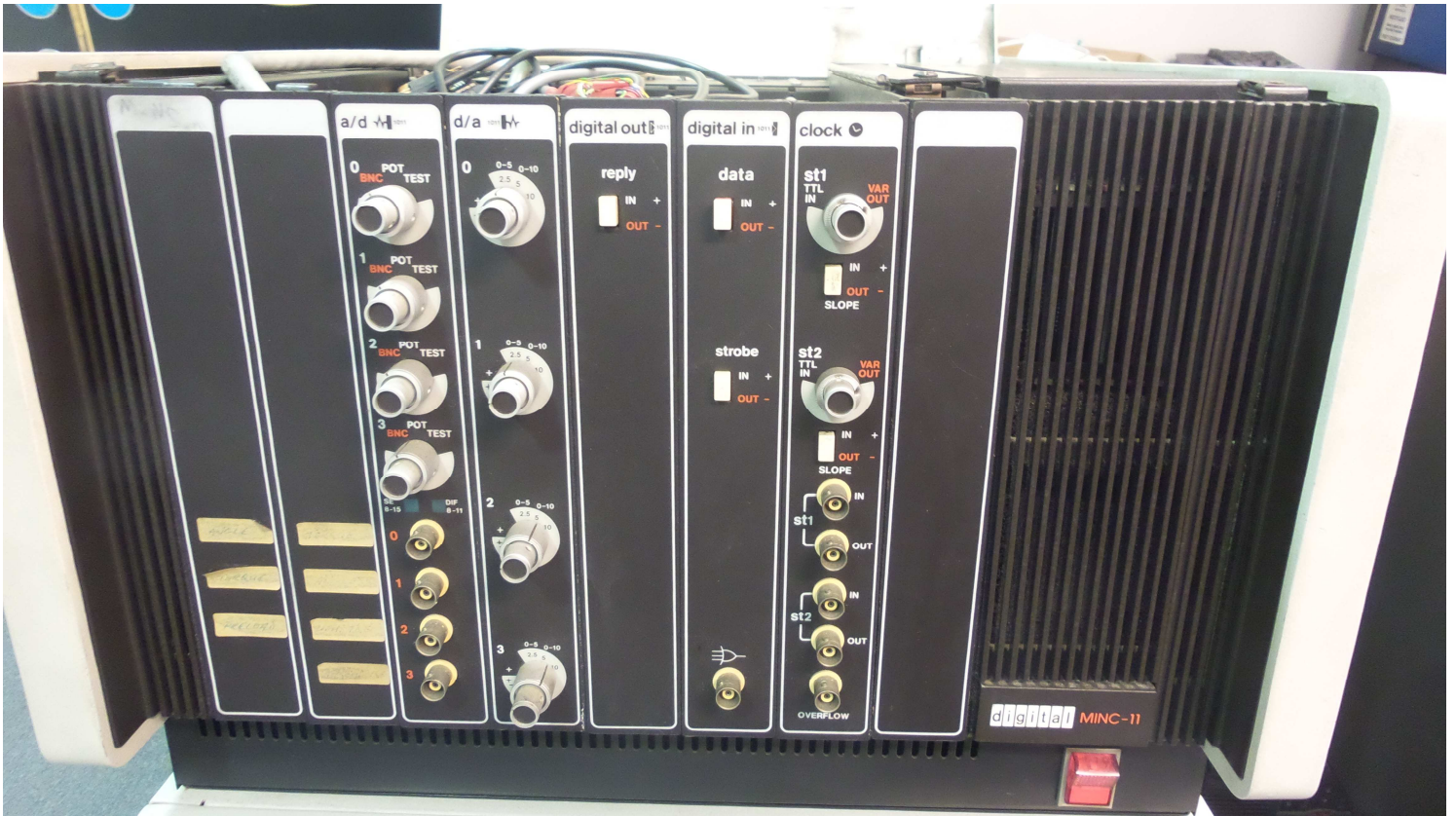
Figure 3: MINC-11 front panel
