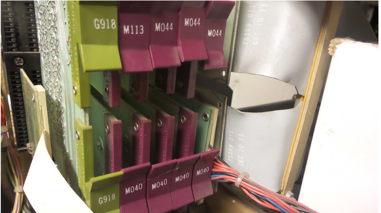
Figure 40: PC04 paper tape unit logic modules
