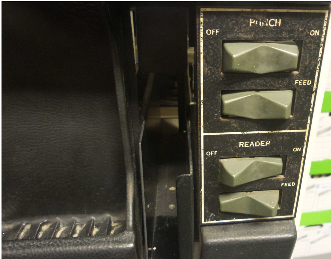
Figure 32: PC04 paper tape unit control panel
