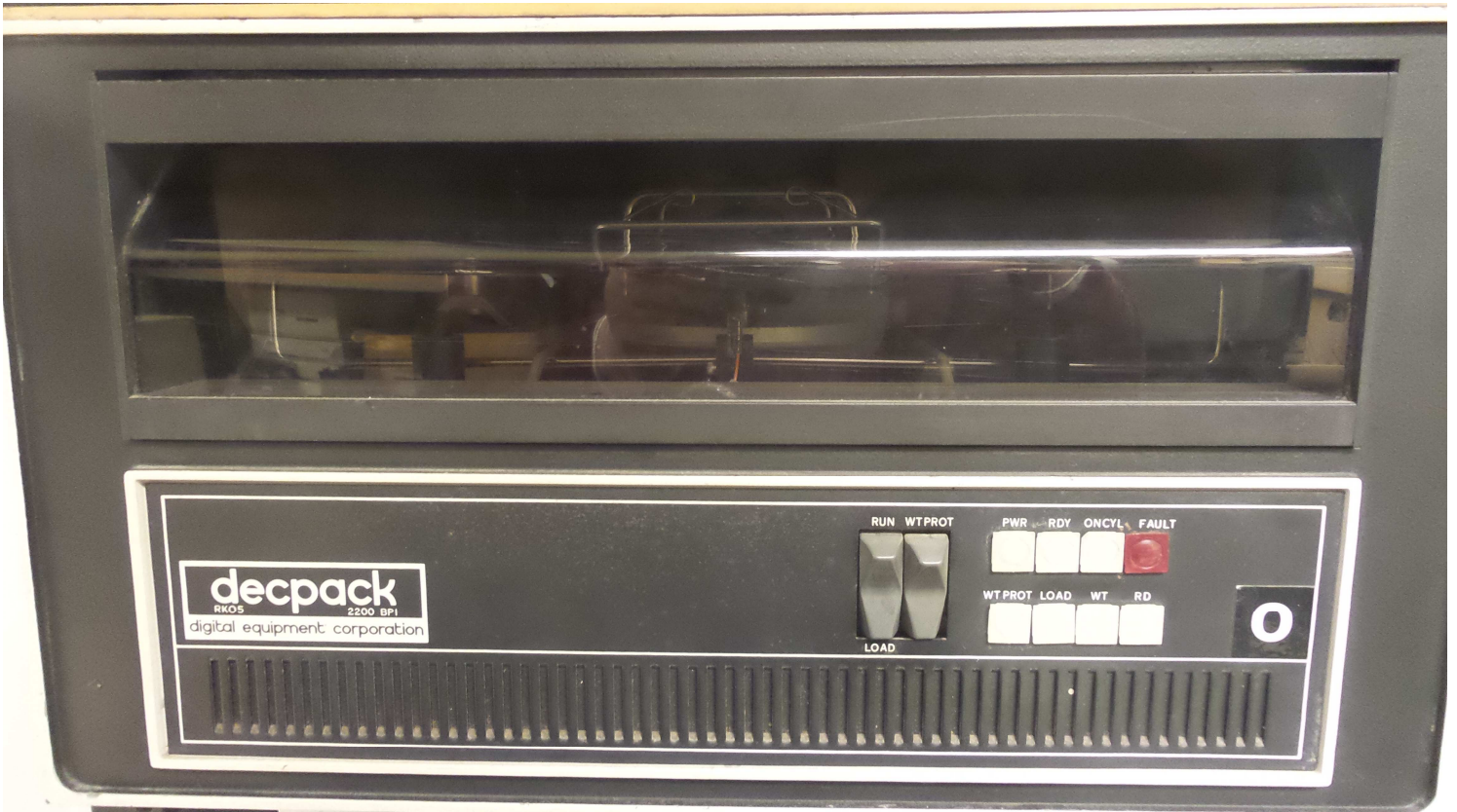
Figure 20: RK05 disk drive front view
