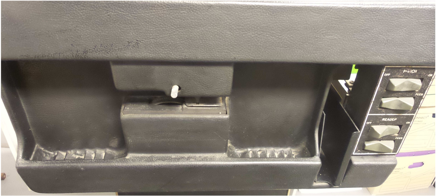
Figure 30: PC04 paper tape unit front view
