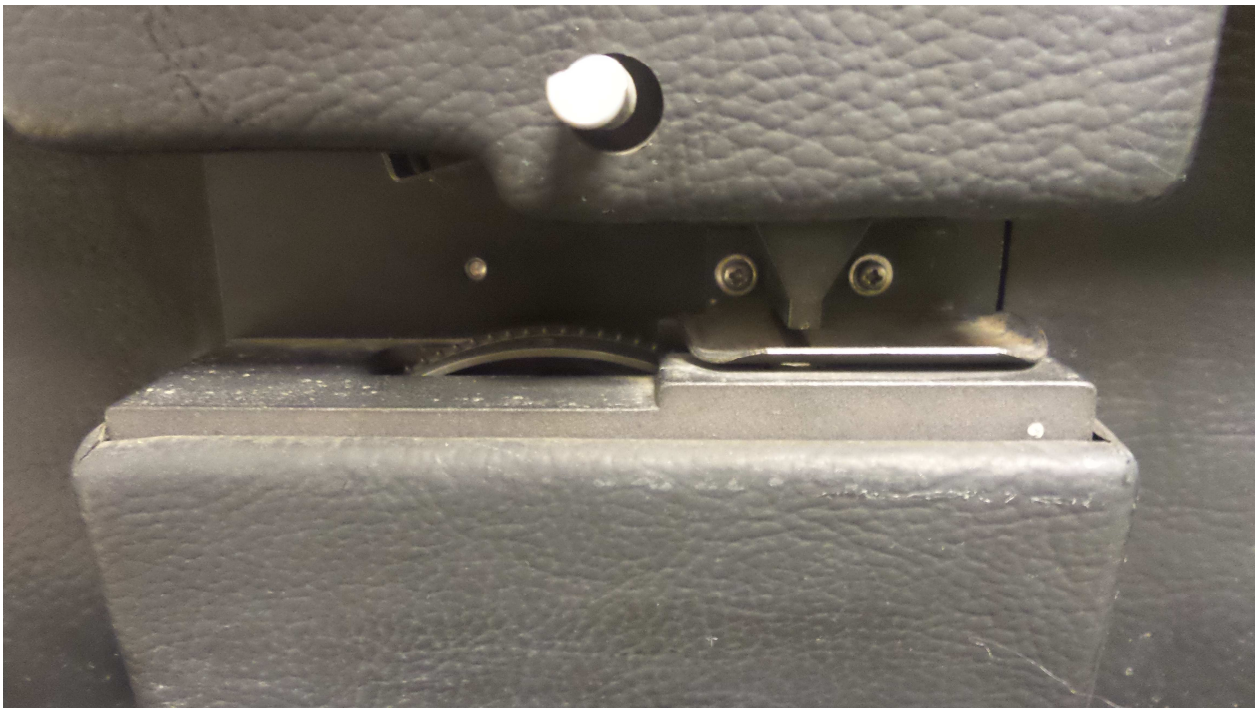
Figure 31: PC04 paper tape unit read head
