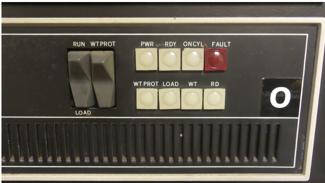
Figure 20: RK05 disk drive front view
