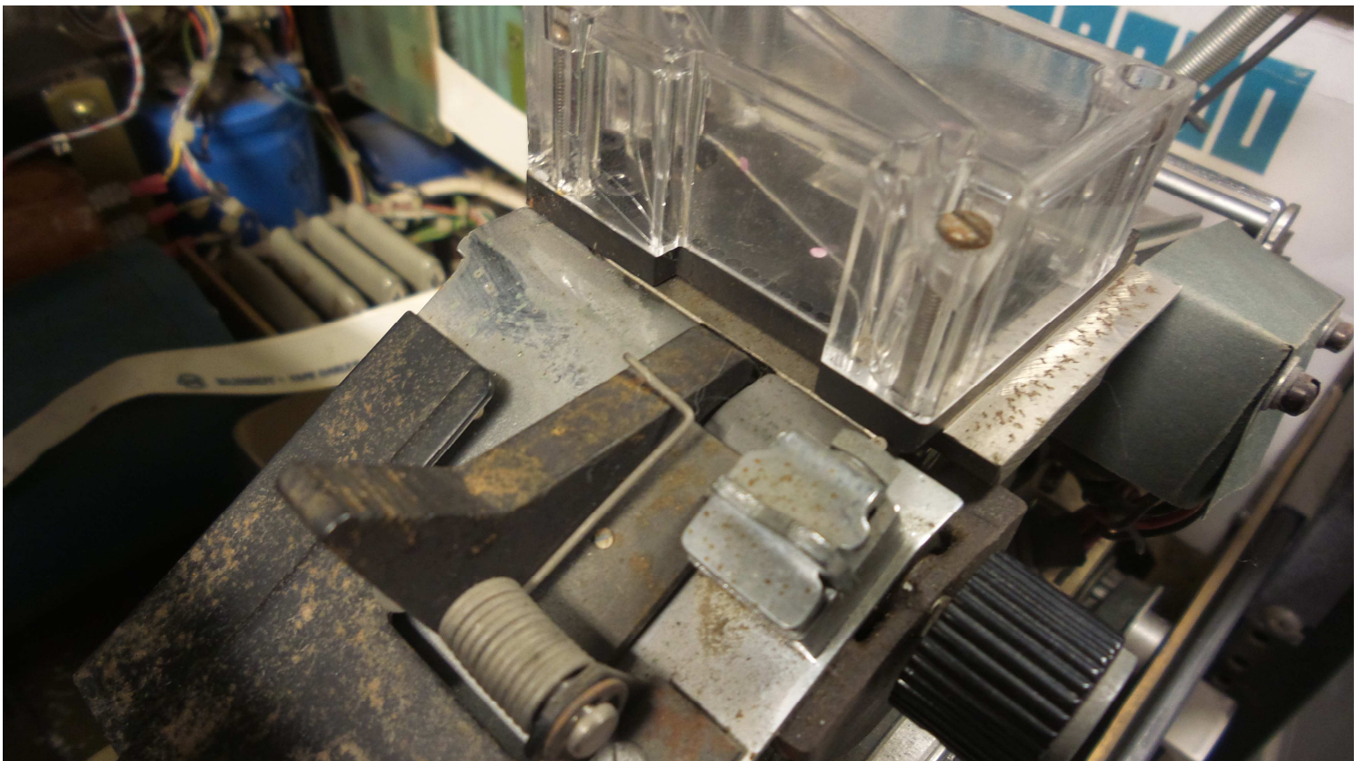
Figure 35: PC04 paper tape unit internal tape punch
