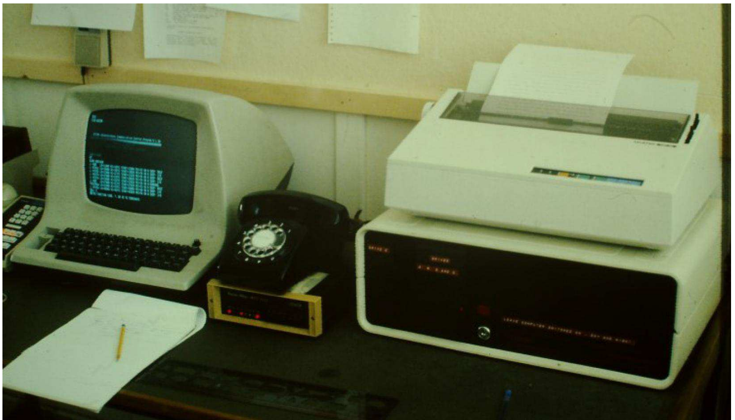
Figure 3: HR-15 printer in action with Comart Communicator, ADM-3A and modem Photograph courtesy Pat O'Byrne
