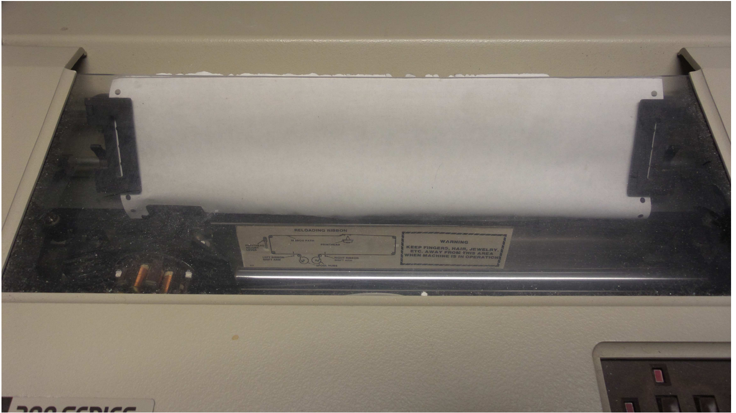
Figure 3: LSI-300 printer tractor-feed carriage, lid closed
