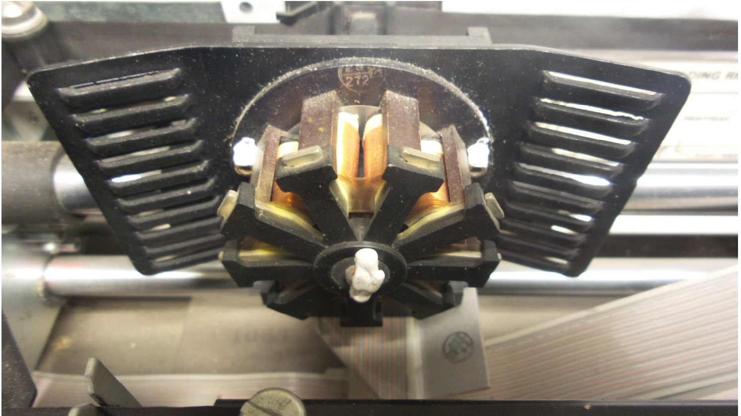
Figure 7: LSI-300 printer, dot matrix head
