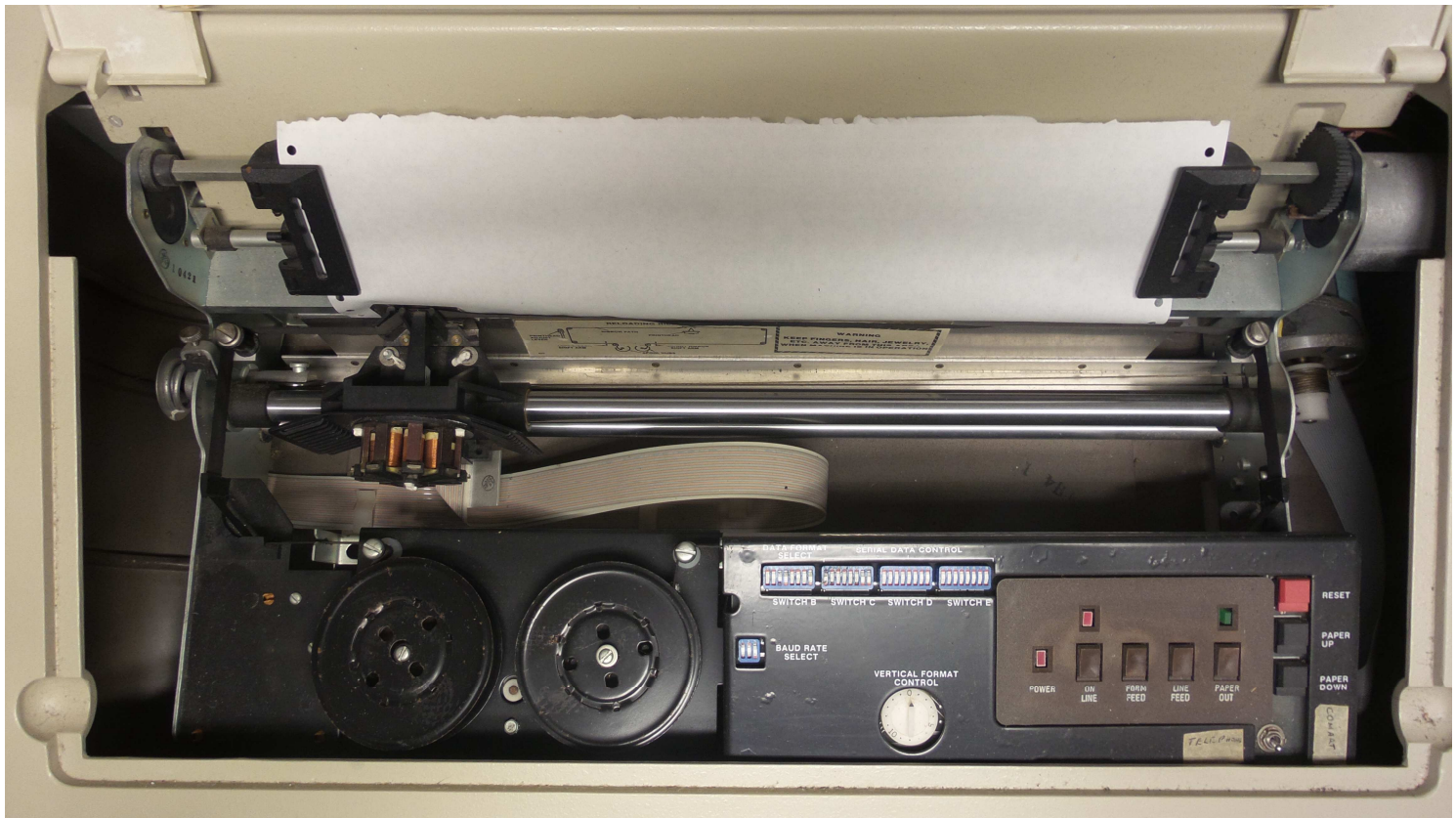
Figure 4: LSI-300 printer tractor-feed carriage, lid open
